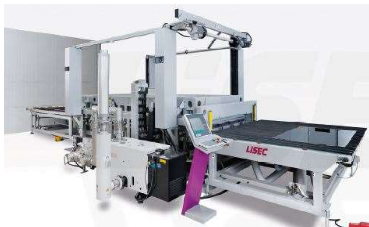
Figure 9 Novel vacuum process laminator
