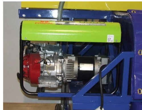
Figure 8 Generator for power supply
