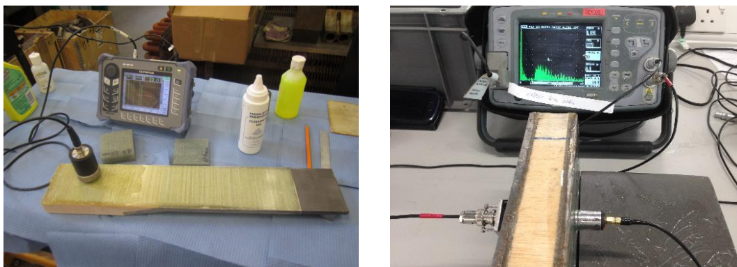
Figure 6 – NDT experiments on hybrid joints.
