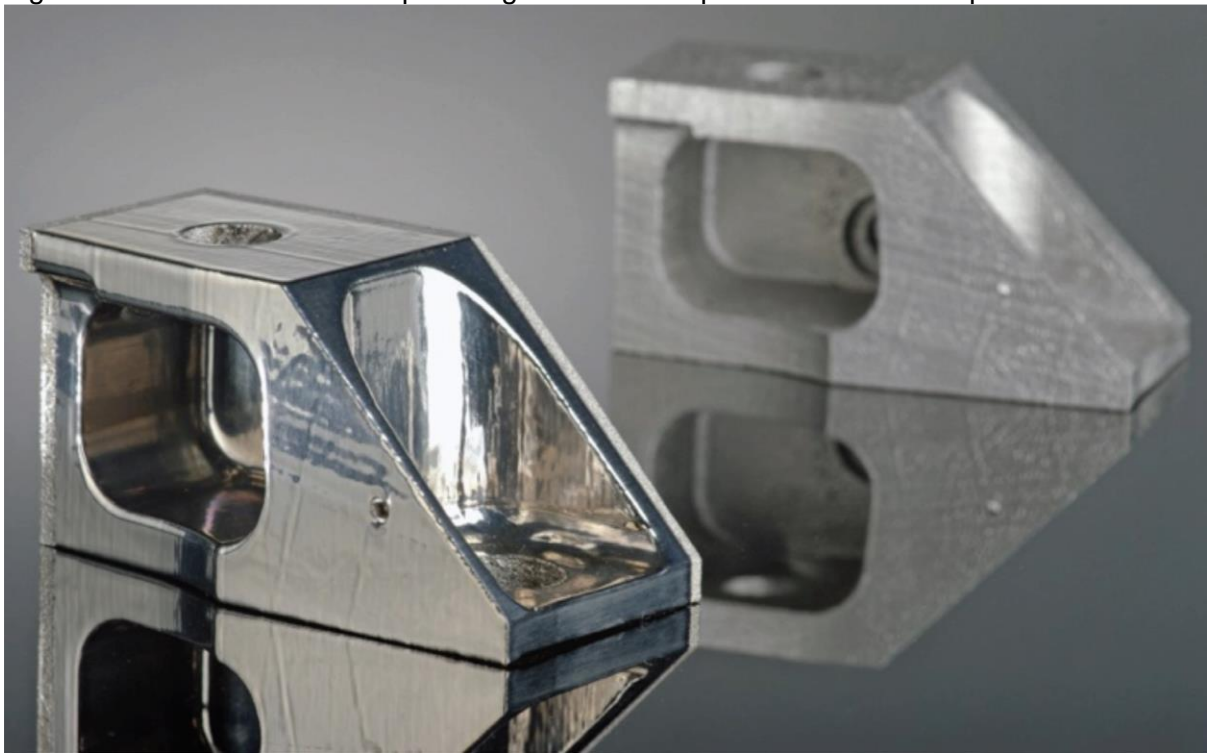
Figure 9 Fraunhofer ILT laser polishing of IN718 compared to Am as built part.
