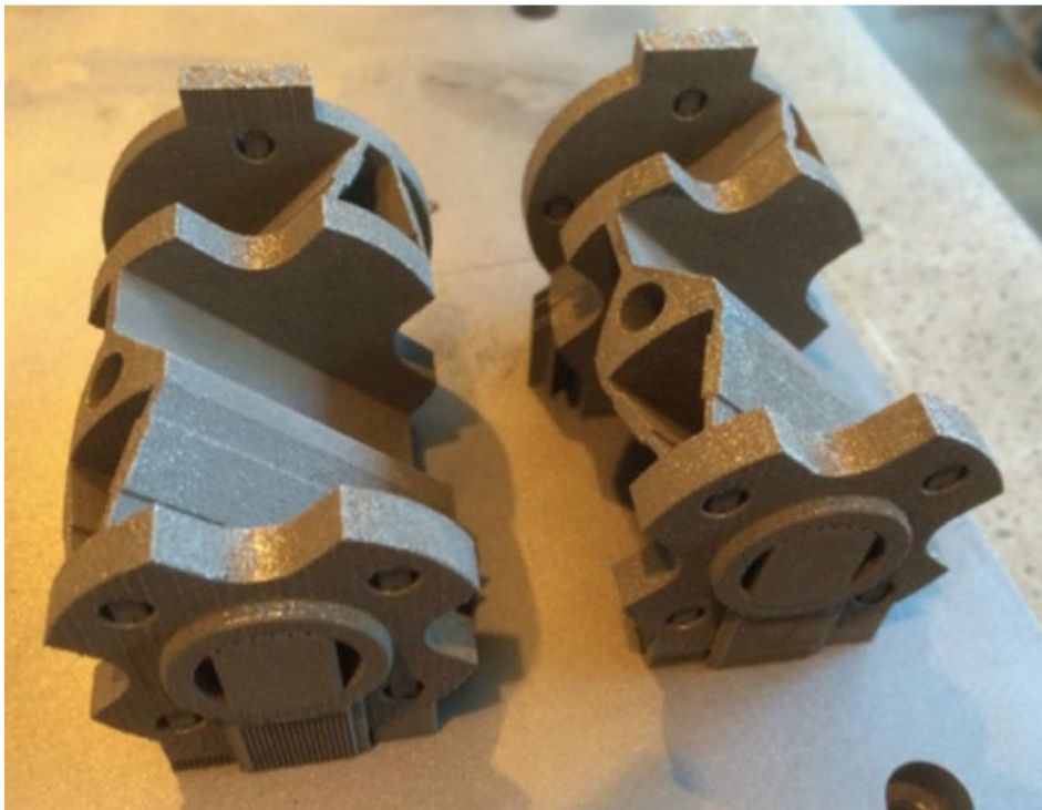
Figure 31 Alloying aluminium and silicon elemental powders by selective laser melting.
