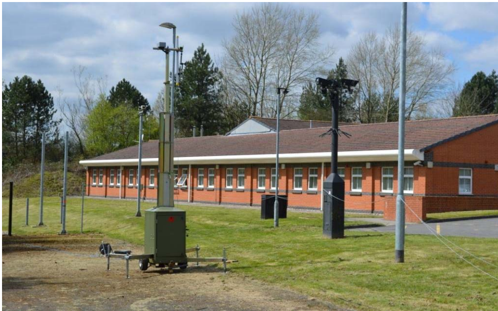
Thermal cameras, visual cameras and radar mounted on mobile poles at the demo site at CAST.
