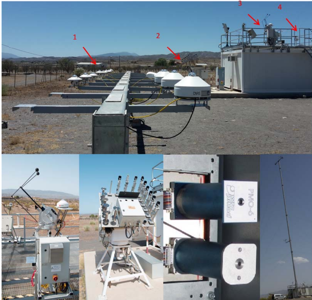
Figure 2. Top: Overview of METAS calibration setup (1: Pyranometer test bench; 2: Pyrheliometers test bench; 3: Black Photon tracker with DHI reference; 4: cloud camera); Bottom left: detail view of Black Photon tracker; Bottom left centre: detail view of pyrheliometer test bench; Bottom right centre: two absolute cavity reference pyrheliometers located in the pyrheliometer test bench's front cabinet; Bottom right: METAS wind mast (WP11).
