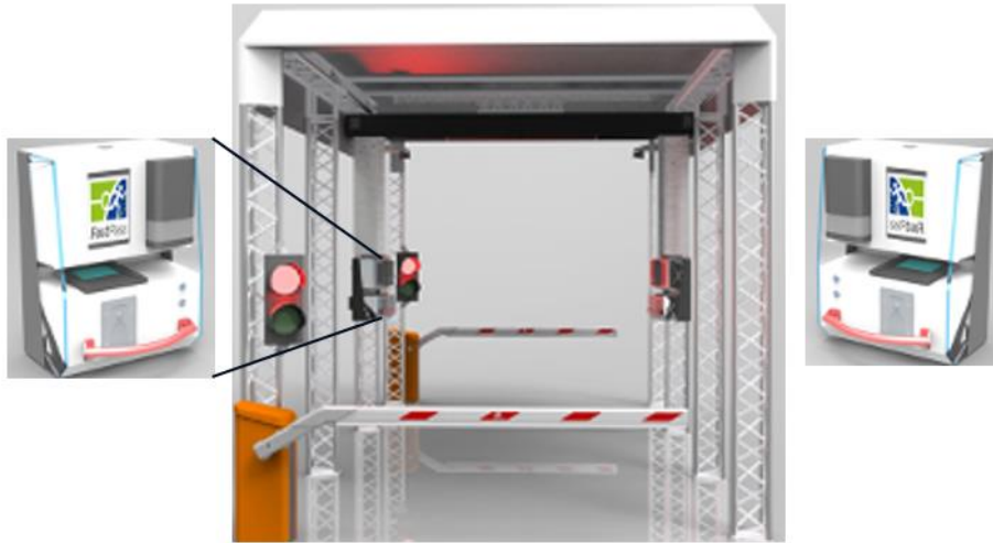
Figure 8: Land border tunnel gate for vehicles and passengers supports 1-4 ABC terminals.
