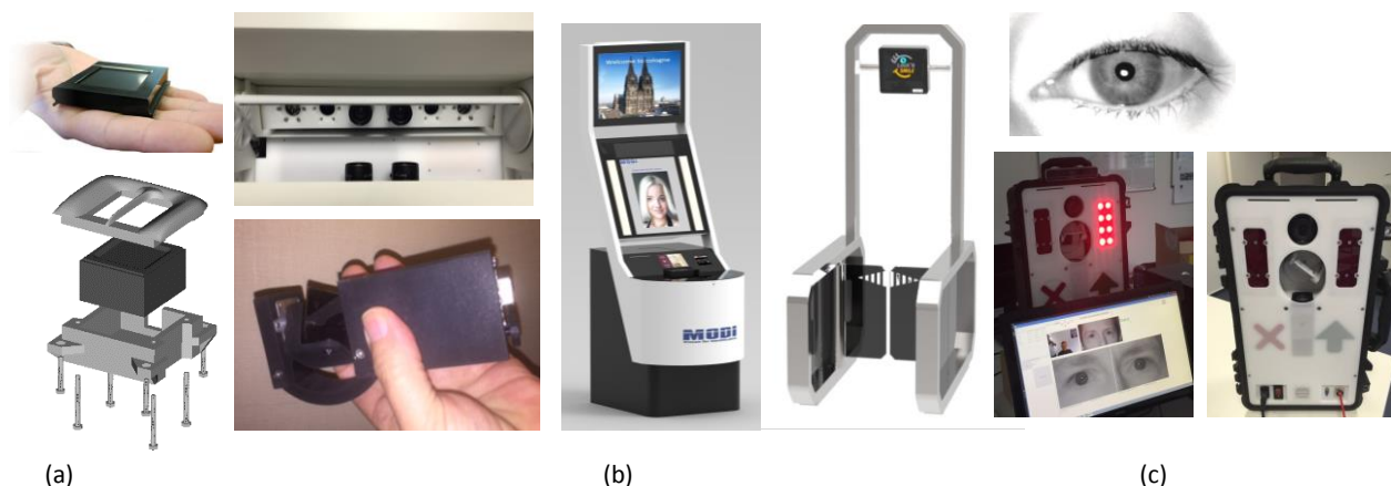
Figure 4: a) Fingerprint finger placement module b) Face recognition system for both kiosk and eGate based on Adomo mirror technology; c) Portable long-distance iris recognition system
