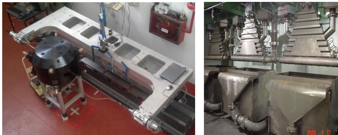
Figure 3: Two applications of accelerator technology: the new AMIT cyclotron for medical isotope production at CIEMAT (Spain) undergoing magnetic field measurements (left) and an industrial water treatment plant using an electron beam in South Korea (right).
