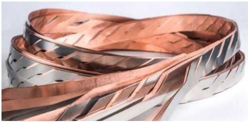
Figure 12: The first Roebel cable produced for EuCARD-2.
