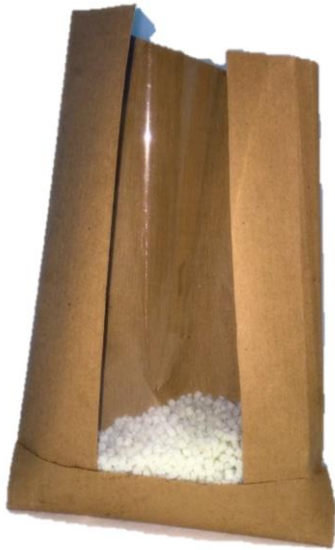
Fig. 7. Paper bag with cellulose film window made by utilizing the 100% biobased adhesive (from SYNPOL biopolymers) for its assembling.
