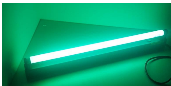
Figure 2 Third batch of FL prototypes using optimized SACS phosphors.
