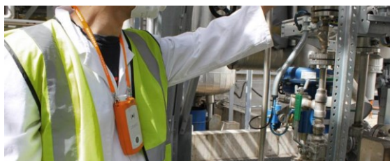
Figure: The NANO BADGE worn as personal sampler during field measurements
