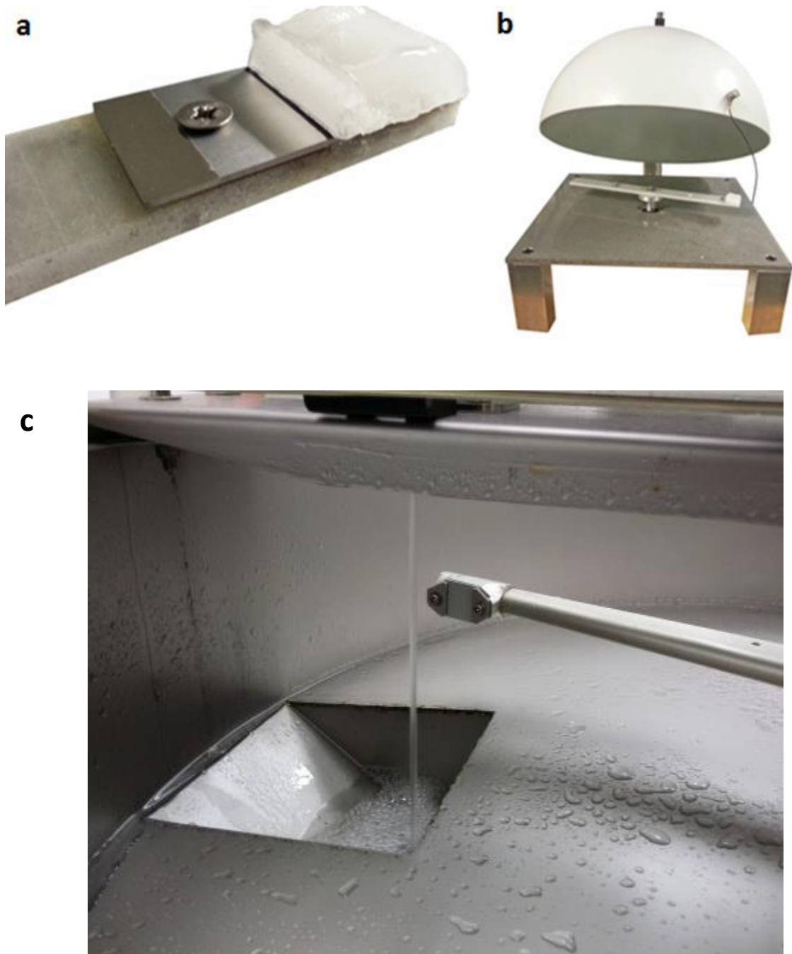
FIGURE 2: (a) Accreted ice on the sample; (b) centrifugal ice adhesion test equipment and (c) water jet erosion test
