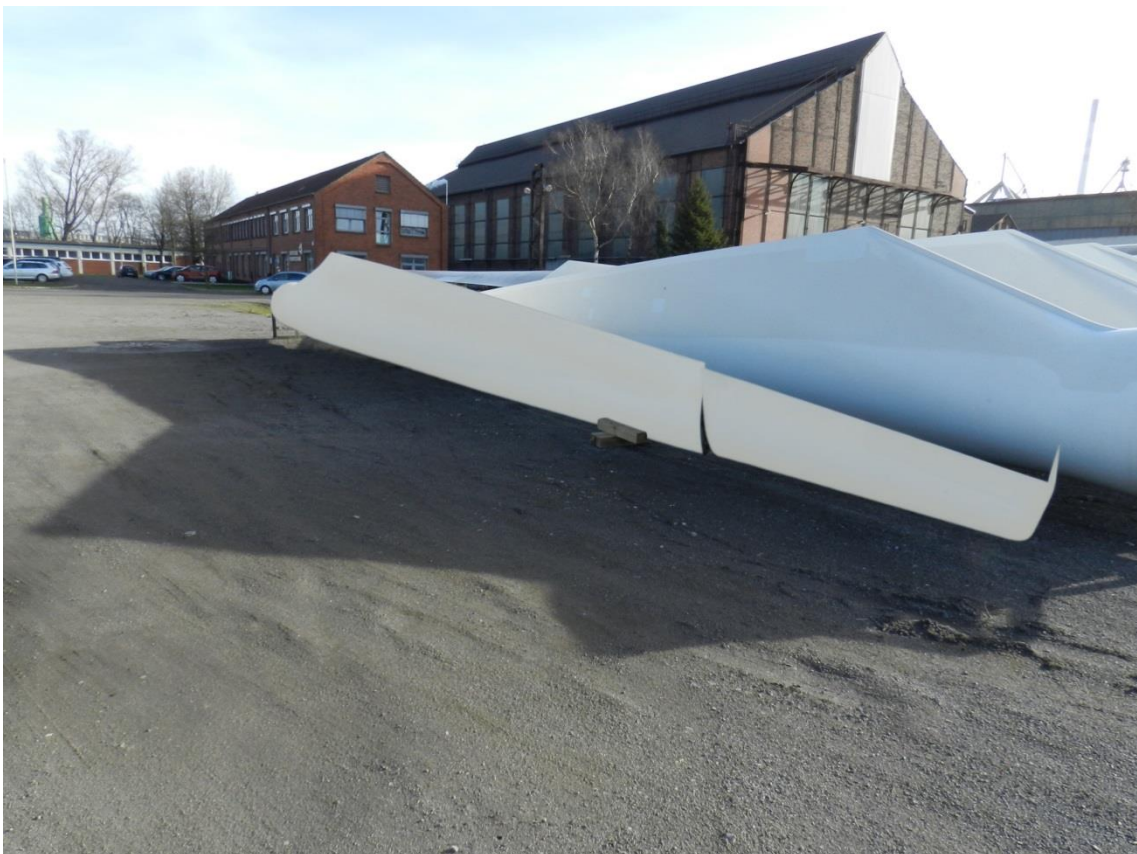
FIGURE 5: Wind blades painted with HBH070, Hydrobond solution
