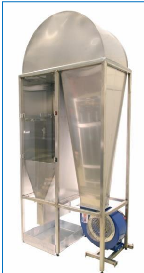
FIGURE 11: Icing wind tunnel at TUT and accreted ice on the sample and centrifugal ice adhesion test equipment
