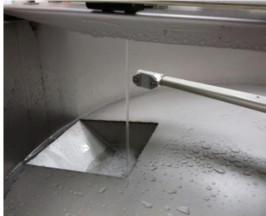
FIGURE 10: Jet erosion test equipment
