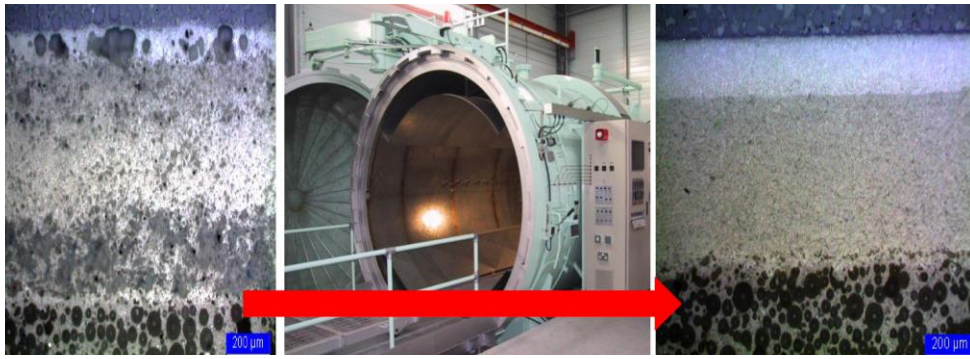
FIGURE 14: Effect of the thermomechanical post-treatment on the coating microstructure (cross-section, optical microscopy, before and after P/T Treatment)
