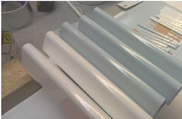
FIGURE 3: Scheme of rain erosion (RE) samples (A); Image of RE samples without coating and coated
