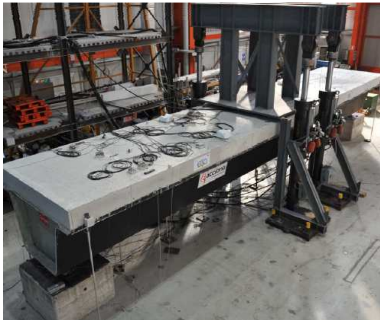
Figure 5. Manufactured beam over test device
