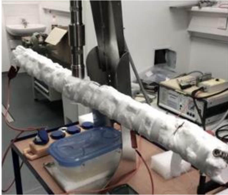
Figure 16: Reactor for post-extrusion sonication
