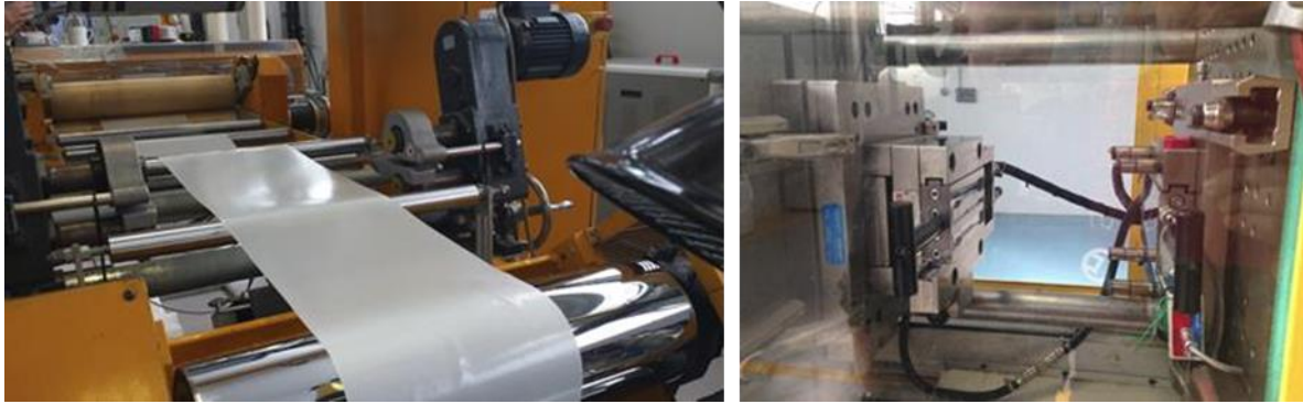
Figure 53: Cast-sheet extrusion and test bar injection of added InnoREX PLA compound
