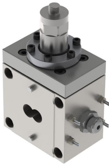
Figure 15: Extruder block for the integration of the ultrasonic device into the twin screw extruder
