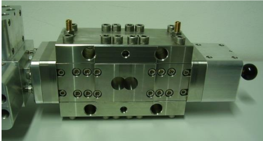
Figure 24: Extruder block designed for microwave injection into the lab-scale twin screw extruder, connected to the shorting plunger on the right and to the E/H tuner on the left (only partly visible) of the 5.8 GHz microwave injection line
