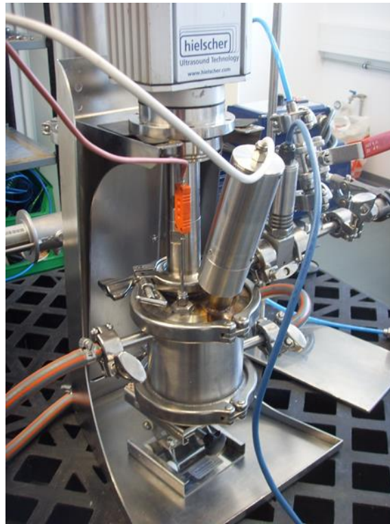
Figure 12: Setup - Ultrasonic batch reactor with pressure sensor and temperature sensor
