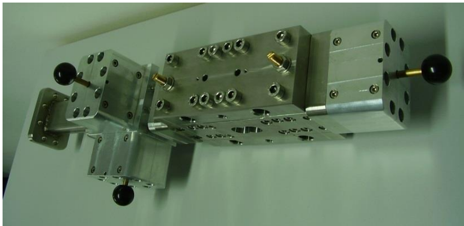
Figure 25: 5.8 GHz microwave injection line including (from left to right) a short piece of R 58 rectangular waveguide, an E/H tuner, the extruder block designed for microwave injection into the lab-scale twin screw extruder, and a shorting plunger
