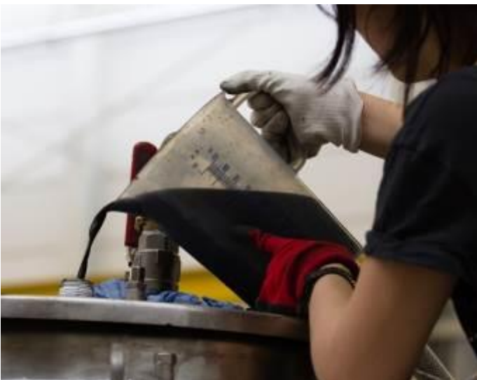
Figure 66: Preparation of the suspension (10 g/L NANOFER STAR and 5 g/L CMC) for the injection into the large scale flume (LSF) at VEGAS (Source: VEGAS, University of Stuttgart, Germany)
