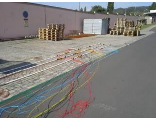
Figure 29: Monitoring system preparation – micropumps and arrays for magnetic susceptibility measurement were prepared (Source: AQUATEST a.s., Czech Republic)
