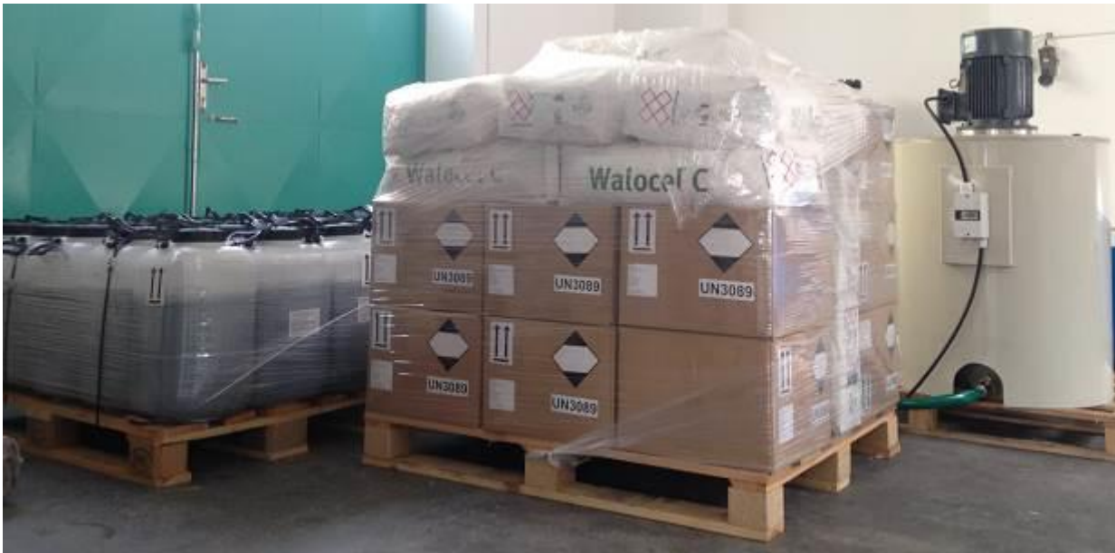
Figure 50: NANOIFER slurry stored in plastic barrels on the left, NANOIFER STAR dry powder placed in a cardboard covers in the middle and a dispersing technology on the right (Source: NANOIRON s.r.o., Czech Republic)
