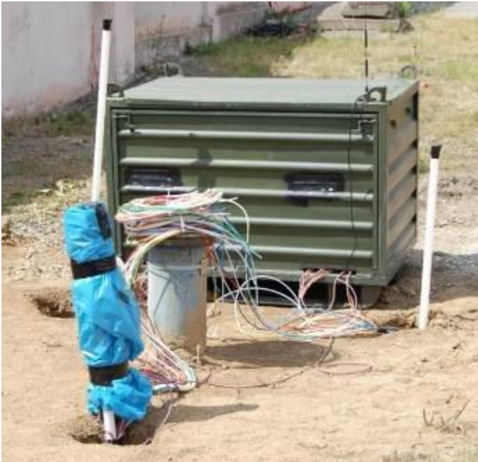
Figure 57: Heads of monitoring arrays for in situ susceptibility measurement (on Ústí nad Labem pilot site) connected to measuring hardware in protective box) (Source: VEGAS, University of Stuttgart, Germany)
