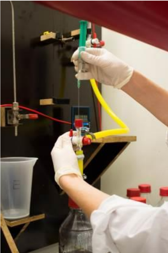
Figure 67: Sample analysis during the injection of NANO FER STAR into the large scale flume (LSF) at VEGAS (Source: VEGAS, University of Stuttgart, Germany)
