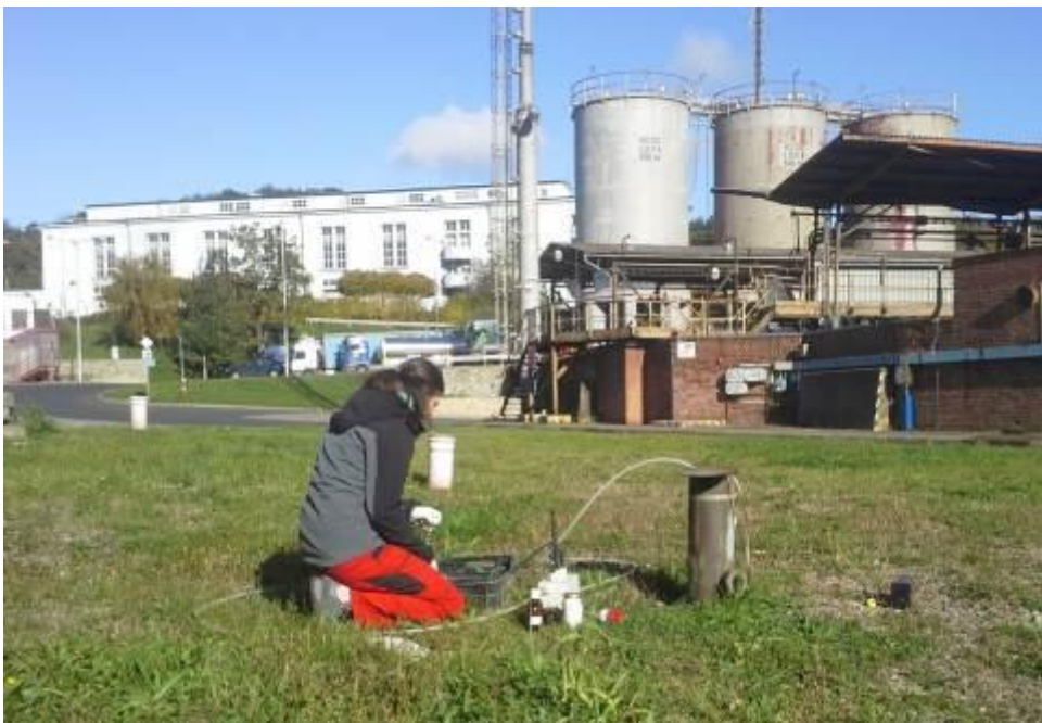
Figure 24: Taking samples for microbiological analysis at Spolchemie (Czech Republic) site after NANO FER STAR injection (Source: Technical University of Liberec, Czech Republic)
