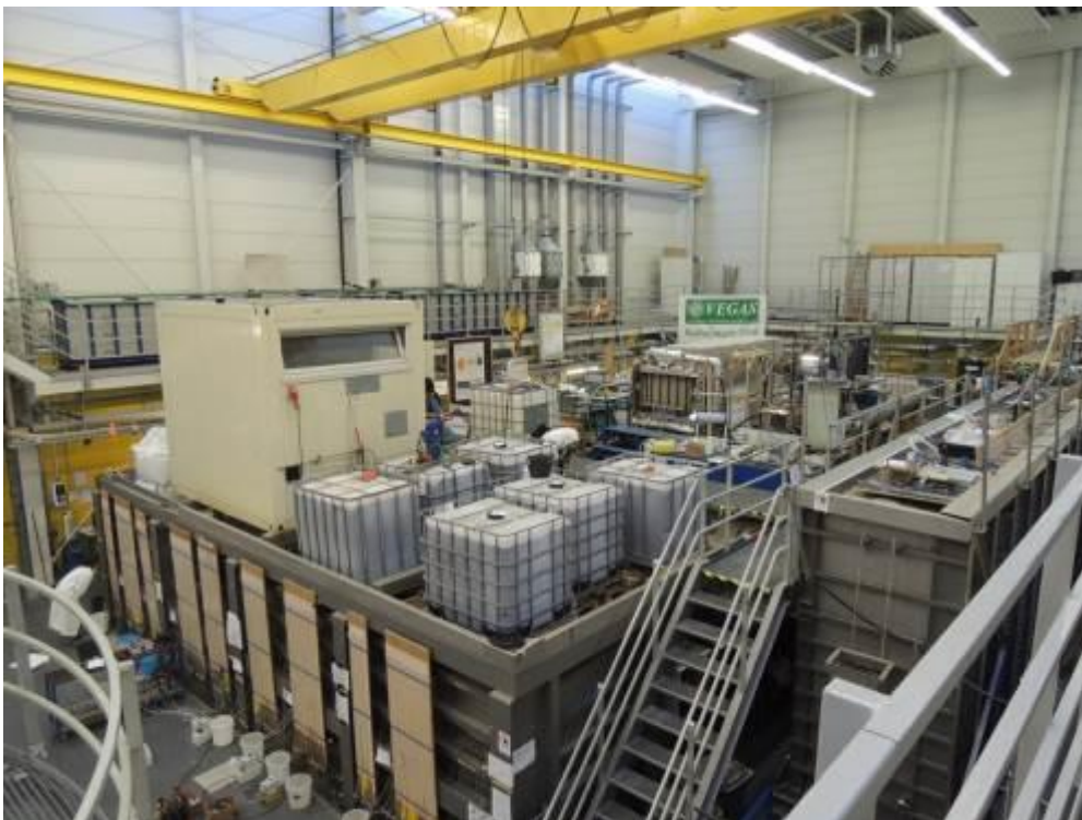
Figure 62: Injection of HMGU iron oxide nanoparticles into the VEGAS large scale container experiment (LSC) at USTUTT in October 2014. Shown here are the 6 IBCs containing the particle suspension, already in place on top of the model aquifer (notice the sandy surface beneath the containers) (Source: VEGAS, University of Stuttgart, Germany)
