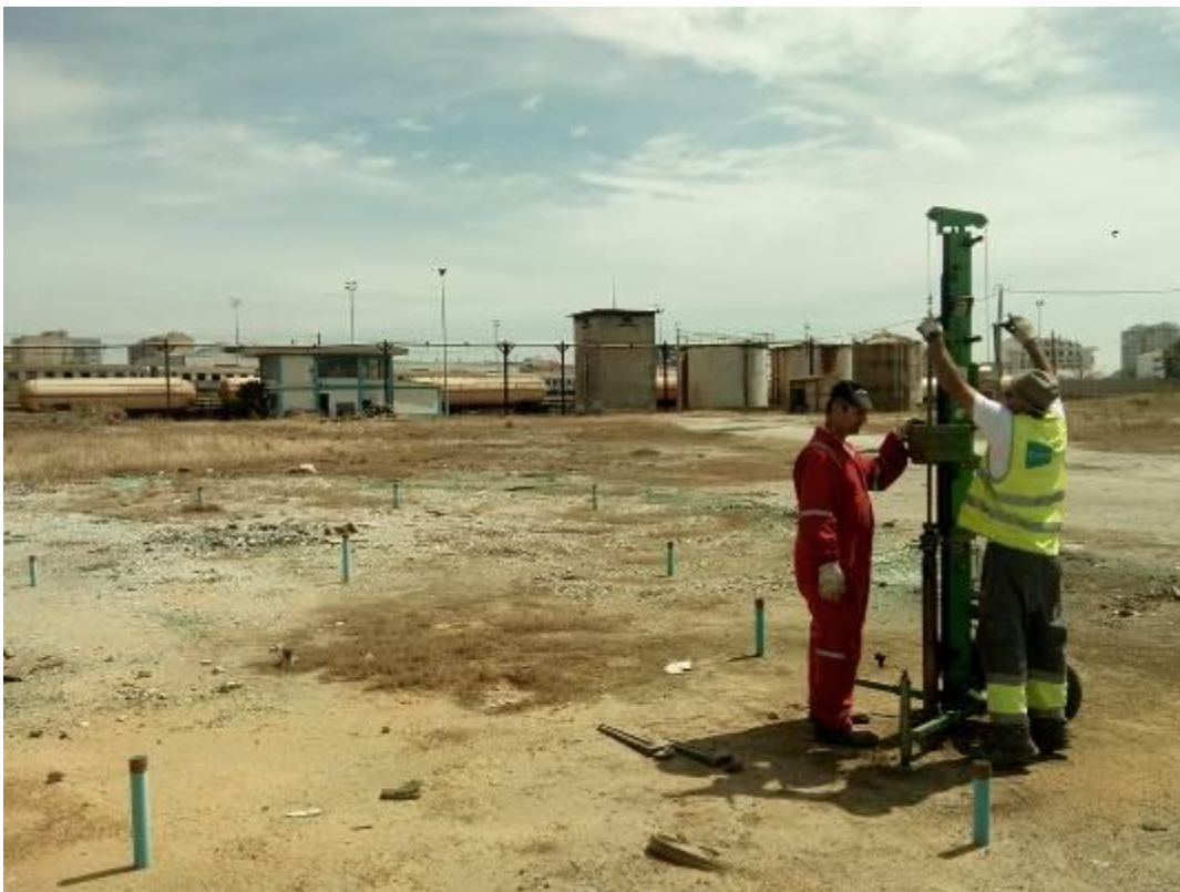
Figure 45: Barreiro site: collection of additional soil samples [18.05.2015] (Source: Geoplano Consultores, S.A., Portugal)
