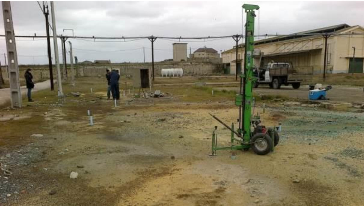
Figure 44: Barreiro site: soil sampling using direct push equipment [20150115] (Source: Geoplano Consultores, S.A., Portugal)
