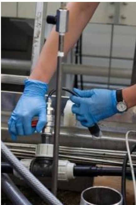
Figure 64: Taking samples of the large scale flume (LSF) experiment during the injection of nZVI (NANO FER STAR) at VEGAS (Source: VEGAS, University of Stuttgart, Germany)
