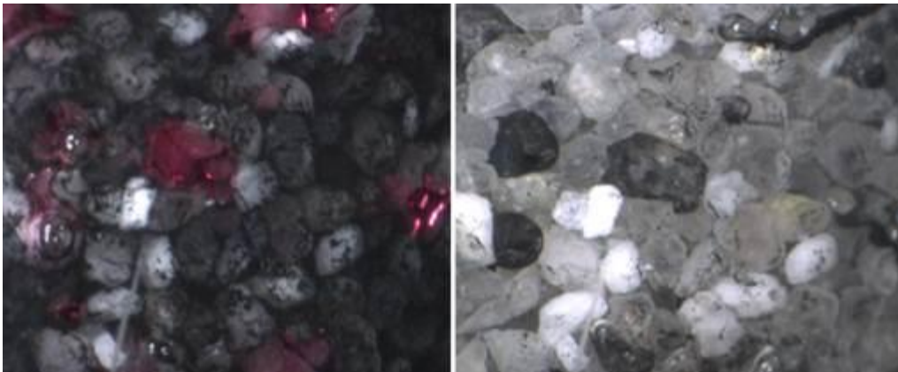
Figure 12: Affinity of Carbo-Iron to (oil-red coloured) to undissolved PCE droplets. Left: Beginning settling during suspension flushing through sediment bed with PCE droplets. Right: Particles remaining attached to droplets even after flushing with distilled water (Source: S. Bleyl, UFZ, Helmholtz-Zentrum für Umweltforschung GmbH, Germany)
