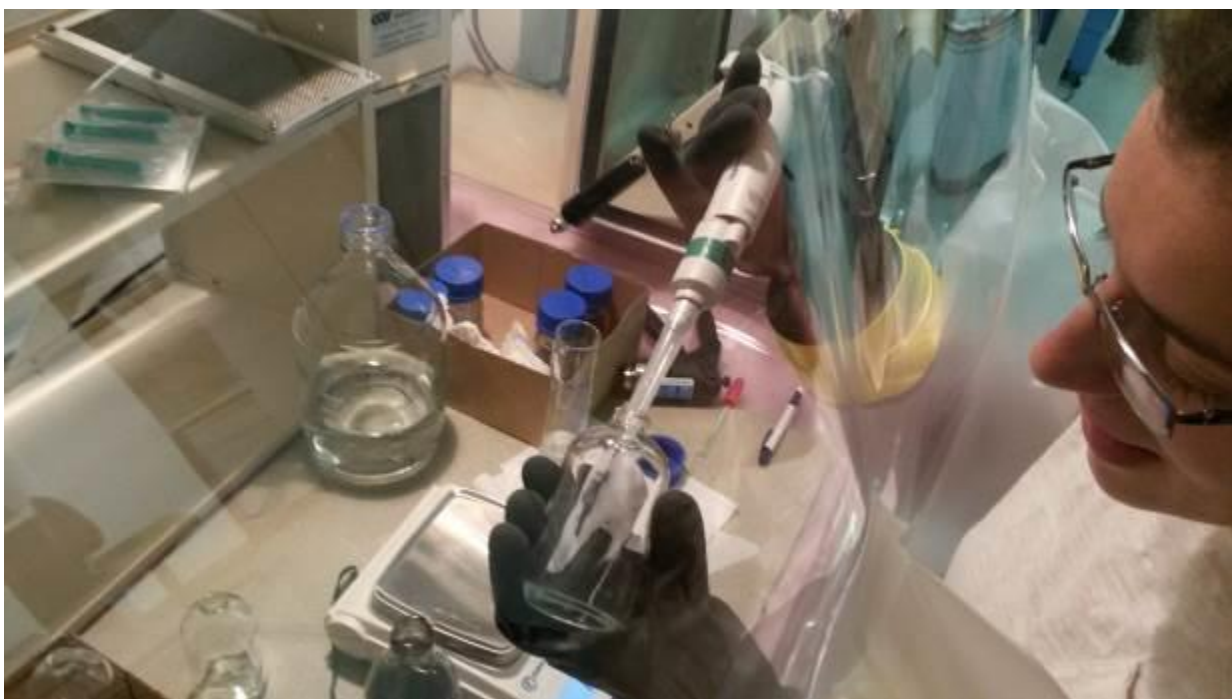
Figure 18: Reactivity tests with FerMEG12 (UVR-FIA GmbH) nanoparticles in a glovebox (Source: Doris Schmid, University of Vienna, Germany)
