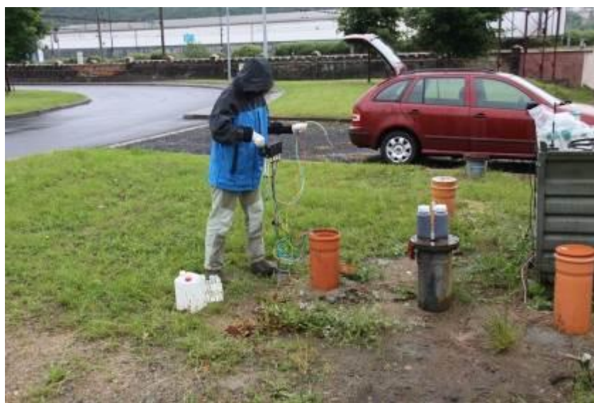
Figure 37: Sampling of nZVI from groundwater at Spolchemie, Site 1, Czech Republic (Source: Ivo Medřík, Palacký University Olomouc, Czech Republic)
