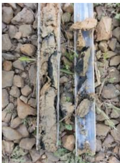
Figure 35: Sampling and on-site analysis (by portable XRF) of nZVI from drill cores at Spolchemie, Site 1, Czech Republic (Source: Jan Filip, Palacký University Olomouc, Czech Republic)
