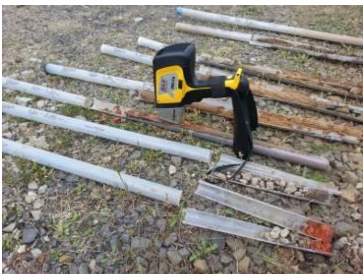
Figure 35: Sampling and on-site analysis (by portable XRF) of nZVI from drill cores at Spolchemie, Site 1, Czech Republic (Source: Jan Filip, Palacký University Olomouc, Czech Republic)
