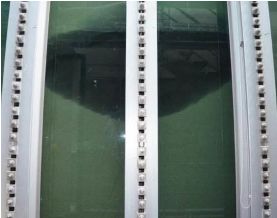
Figure 61: Spreading of Carbo-Iron suspension in the large scale flume experiment (Source: VEGAS, University of Stuttgart, Germany)
