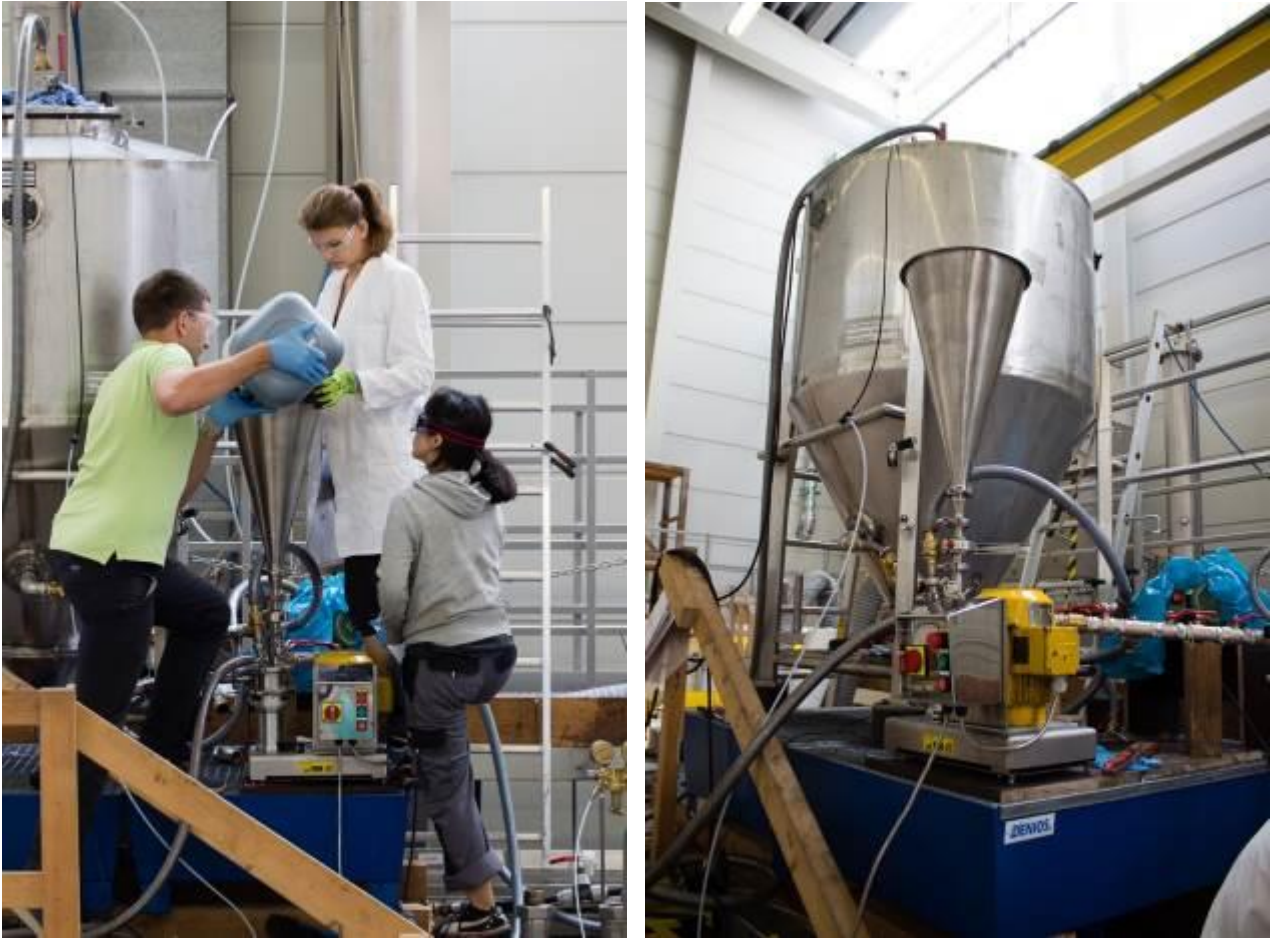
Figure 63: Preparation of the suspension (10 g/L NANO FER STAR and 5 g/L CMC) for the injection into the large scale flume (LSF) at VEGAS (Source: VEGAS, University of Stuttgart, Germany)
