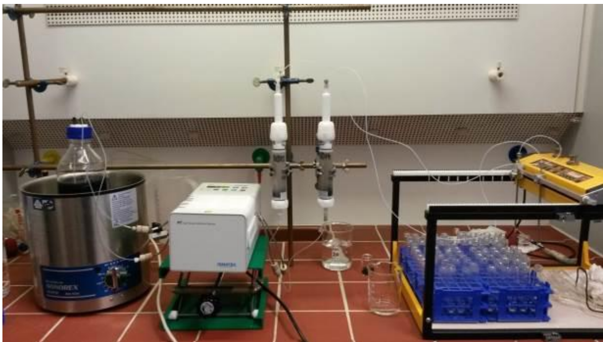
Figure 17: Nanoparticle mobility test at UNIVIE (Source: Doris Schmid, University of Vienna, Germany)
