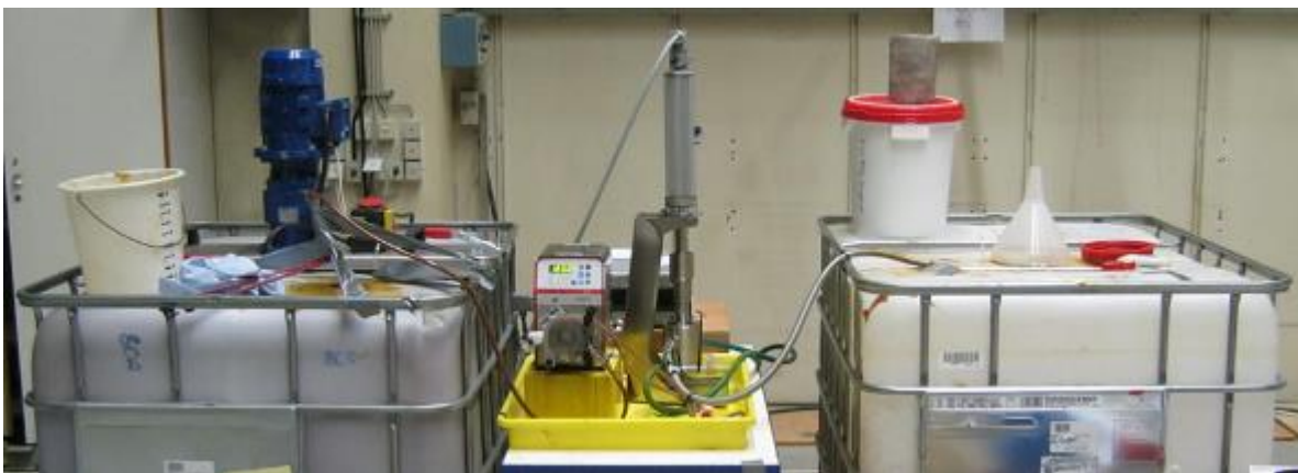
Figure 54: Made in Germany - Industrial scale production of Nano-Goethite nanoparticles. Nanoparticulate iron oxide colloid production at HMGU in preparation of the VEGAS large scale container experiment. One cubic meter of suspension is produced from a commercial precursor by multiple industrial, water-cooled ultrasonification steps and subsequent coating with organic electrosteric stabilizers (Source: Helmholtz Zentrum München, Germany)
