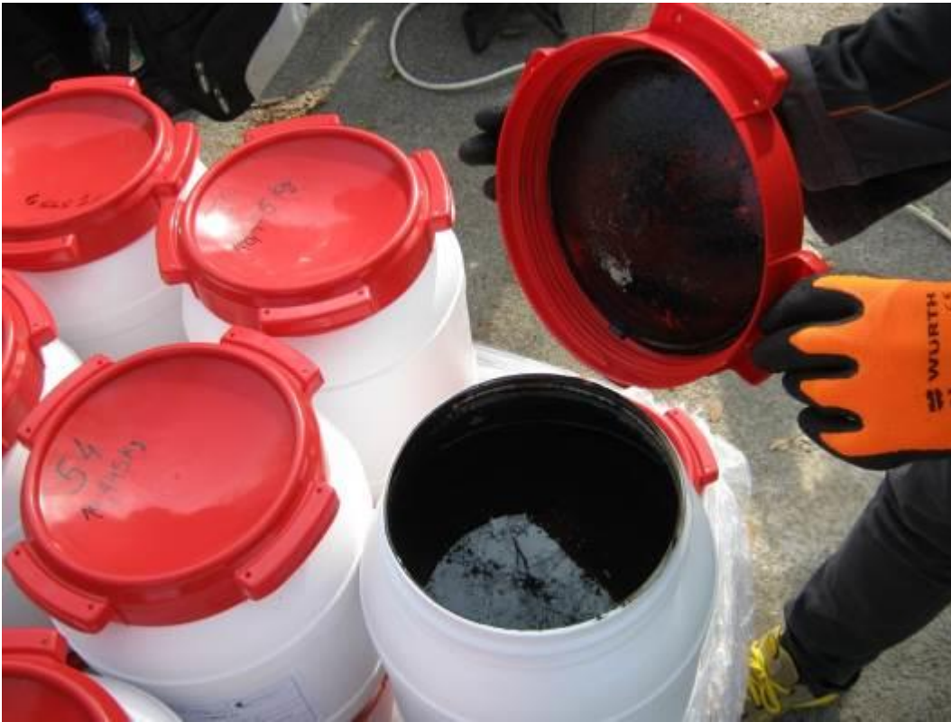
Figure 69: Injection of FerMEG12 (nZVI) into the Solvay site (Source: VEGAS, University of Stuttgart, Germany)
