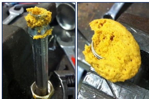
Figure 2.7 Dough-like catalyst right after opening the reactor when no inhibitor was used due to the product residue in the catalyst bed
