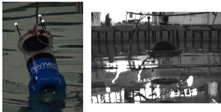
Figure 10. Tubular moored Poly-OWC prototype based on the Sendekia collector in operation at Flowave.
