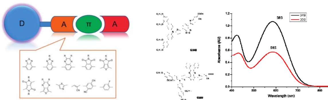
Figure. 4 (Left) Concept and schematic illustration of D-A- \pi -A structure. (Right) UV-VIS spectrum of two prototypical blue colored D-A- \pi -A sensitizers.
