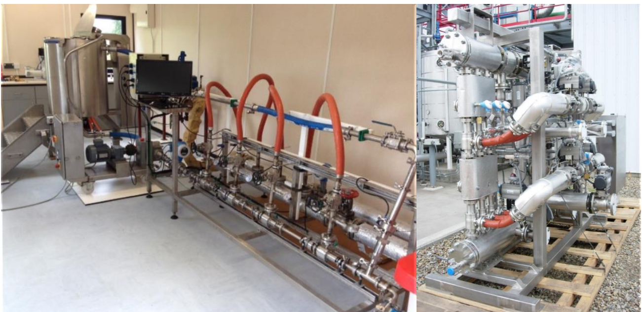
Figure 12. Small (left) and large (right) rig of the Soniqueflo by Cellulac, used for cell cracking
