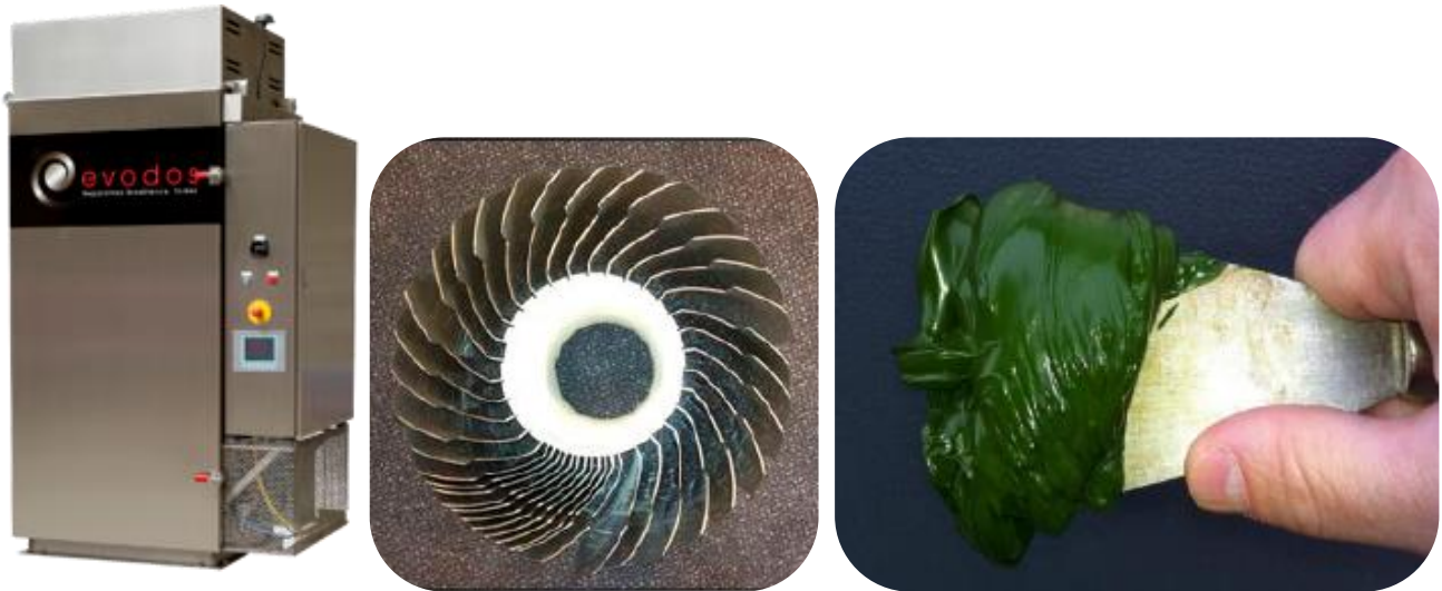
Figure 11. Left: The Evodos 25 with automated discharge system; Middle: the spiral plate technology; right: the harvested paste
