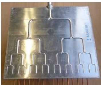
a) stamped single 1-to 16 element distributor
