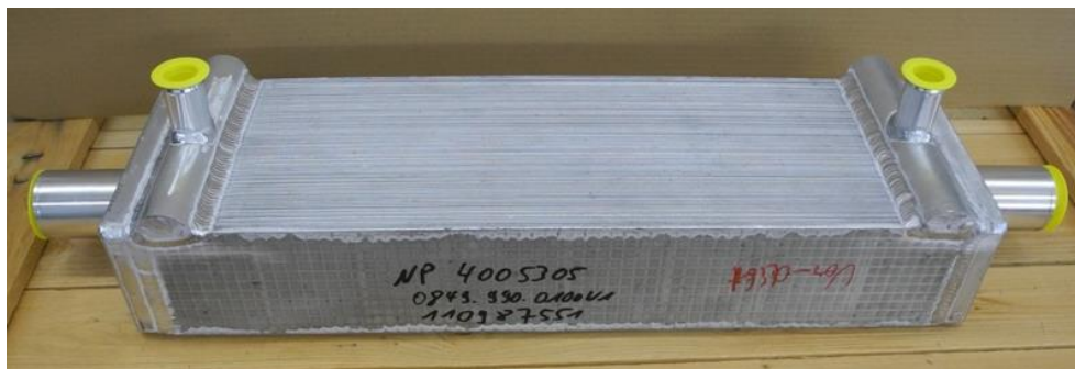
Figure 23: Photo of condenser
