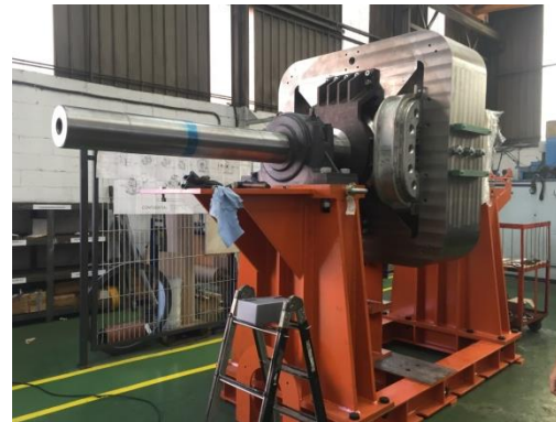
Figure 38. Picture of the assembly of the electromagnetic elements in the shaft and bench
