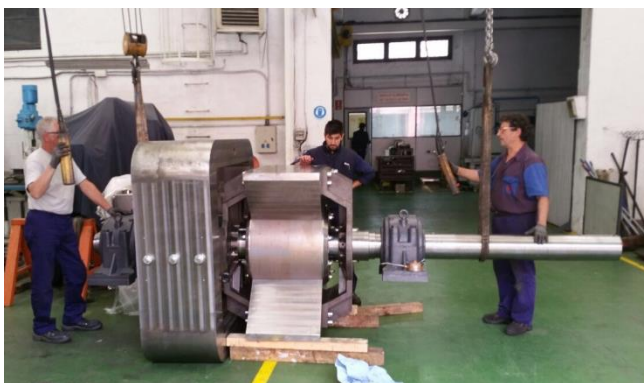
Figure 38. Picture of the assembly of the electromagnetic elements in the shaft and bench
