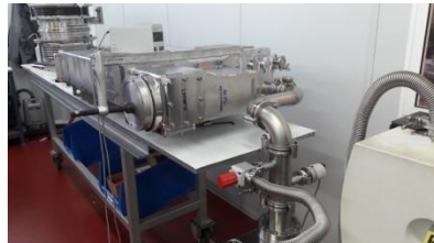
(c) vacuum test after welding
