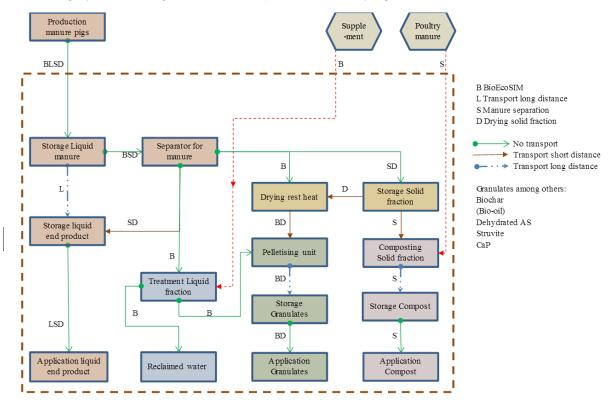
The comparative sustainability impact assessment also considered the alternative setup of BioEcoSIM without pyrolysis and with soil improver rather than biochar as product from the solid fraction processing.
