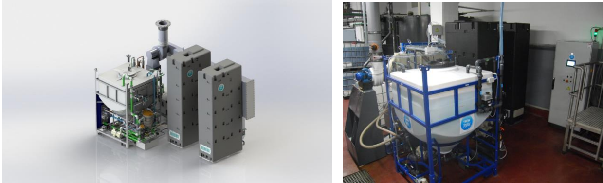
Figure 6: The 2 MHD evaporation units and its control system implemented in the ECOWAMA pilot plant
