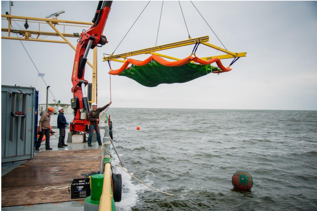
Figure 23. The edgeweighted artificial seagrass mat and lifting frame during deployment.
