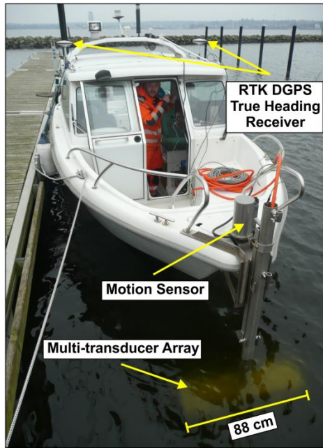
Figure 7: Setup of acquisition hardware with 3D sub bottom profiler transducer array, motion sensor and dual-antenna RTK DGPS mounted on the survey boat
