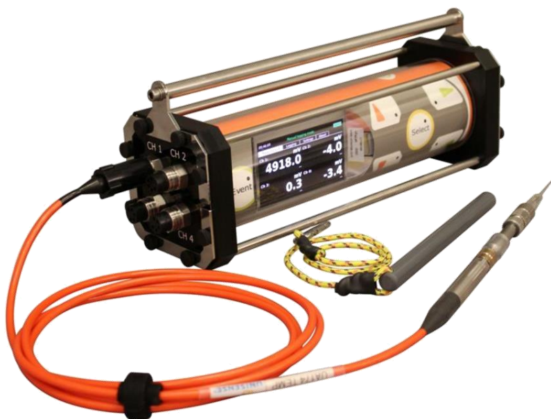
Figure 10: Data logger for characterising environmental parameters in sediments. The logger has four channels and are being developed to measure sulphide, pH, redox potential and dissolved oxygen.
