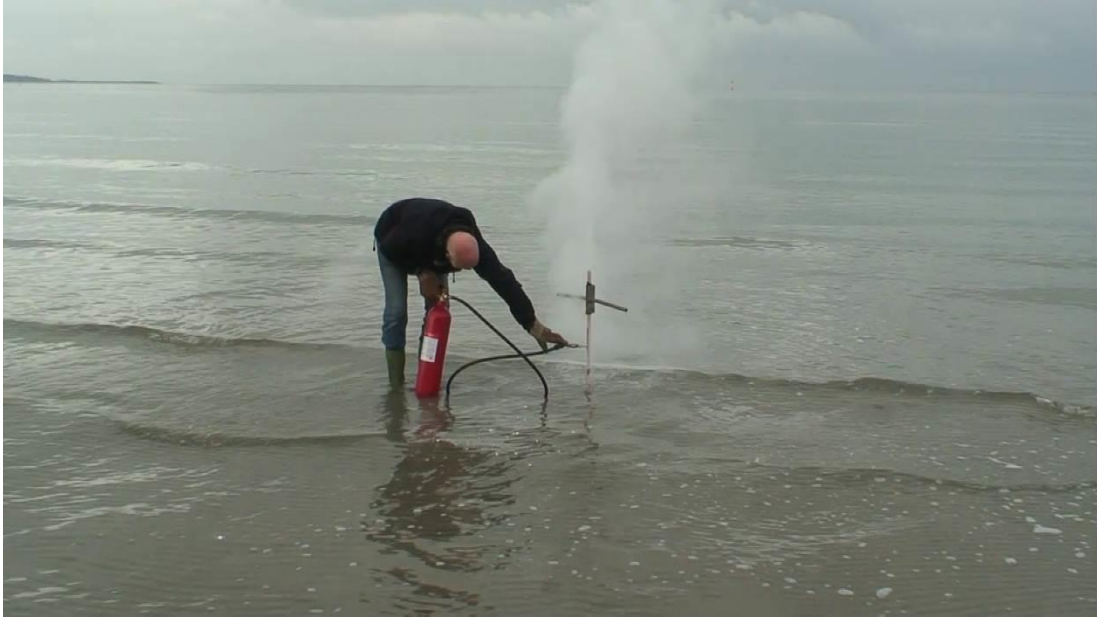
Figure 20. Freezing system for sandy sediments showing excess carbon dioxide being vented
