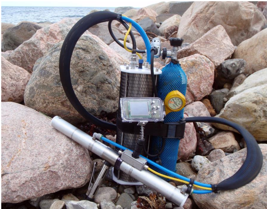
Figure 16: The diverheld underwater wood tester (WP4UW)
