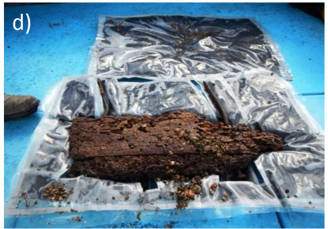
Figure 22. Use of carbon fibre impregnated with treated with cured epoxy-time enclosed in a plastic vacuum bag.
