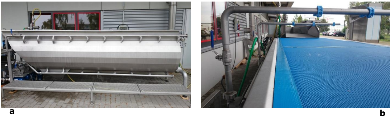
Figure 6 Washing system: a) Washing unit and b) Double spraying system
