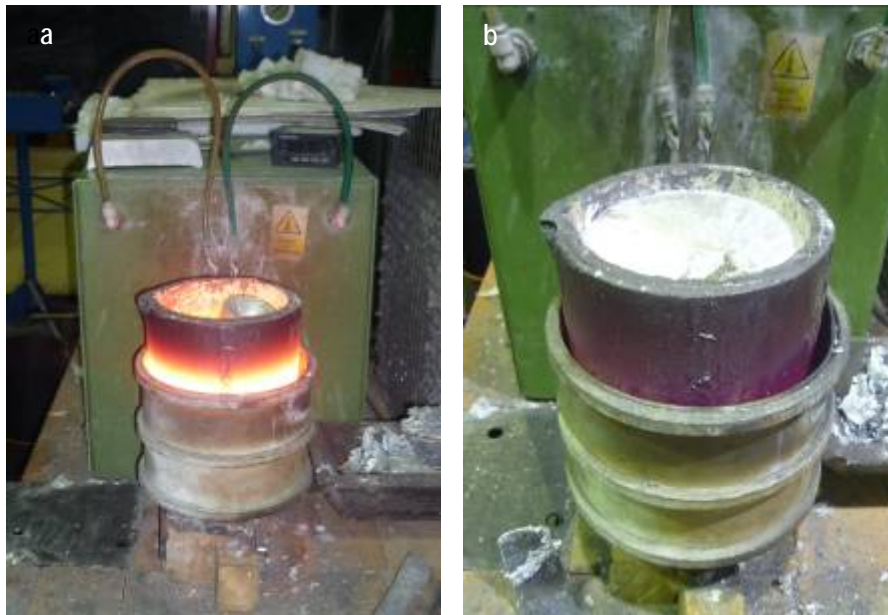
Figure 3: (a) Melting of pure Al in the induction furnace, (b) molten Al in the SiC crucible.
