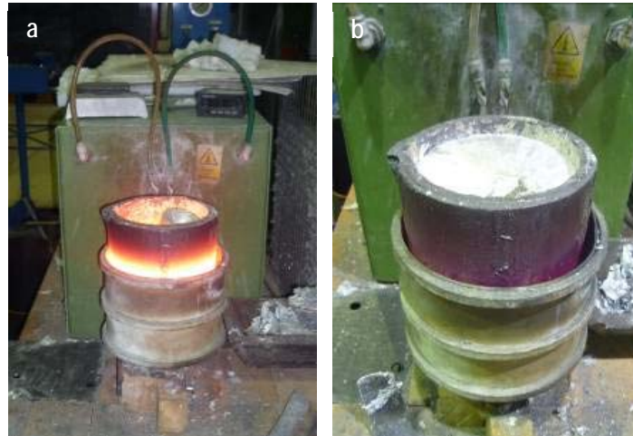
Figure 1. (a) Melting of pure Al in the induction furnace, (b) molten Al in the SiC crucible.
