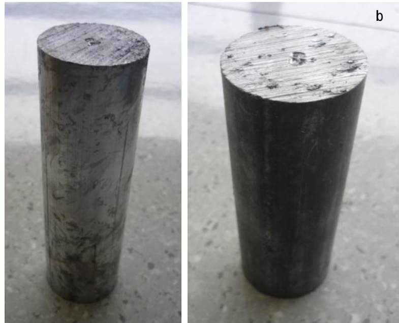
Figure 6: Extruded cylinders in the (a) as-extruded and (b) extruded + heat treated condition.
