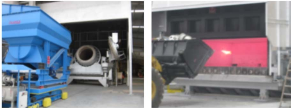
Figure 19. Rotary and reverberatory furnaces used for the production of the final batches of the developed alloys.
