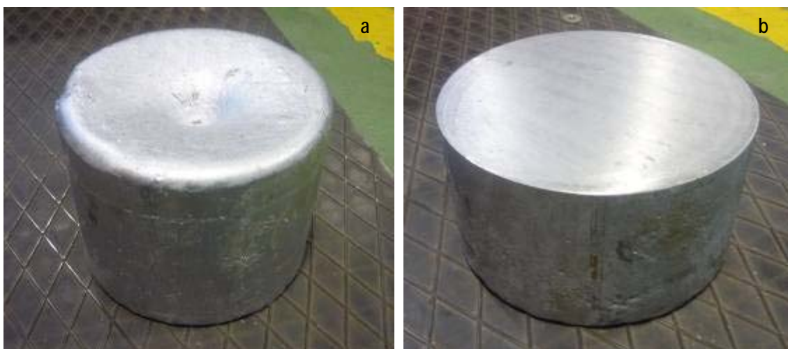
Figure 5: Cast big cylinder (a) after demoulding and (b) after removing the top part.
