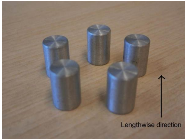
Figure 13. Compression test specimens machined from delivered aluminums
