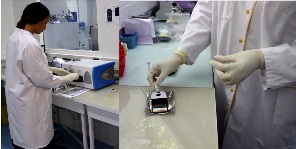
Figure 5. The GeneSpress instrument undergoing user testing. Cartridge insertion into the instrument is shown on the left hand side, the right hand side shows pouring of sample into the cartridge.
