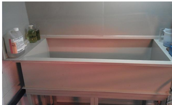
Figure 16 Development Plating Tank
