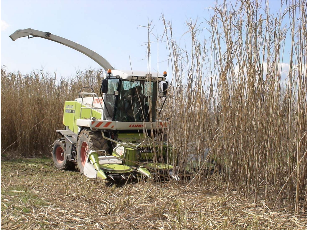
Figure 7 – SPAPPERI. Claas jaguar and kemper head during harvesting operation in northern Italy. Photo by CREA-ING
