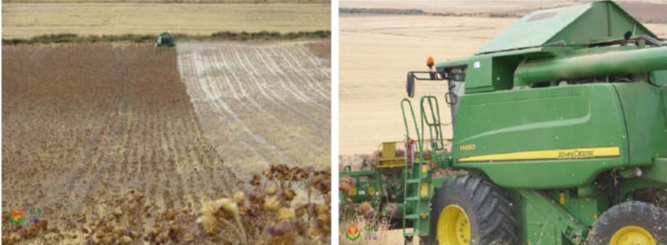
Picture 1 - UPM. Mechanical harvest of seeds of cynara by means of a conventional Jonh Deere W650 harvester with Kemper 206 header. September 2013..
