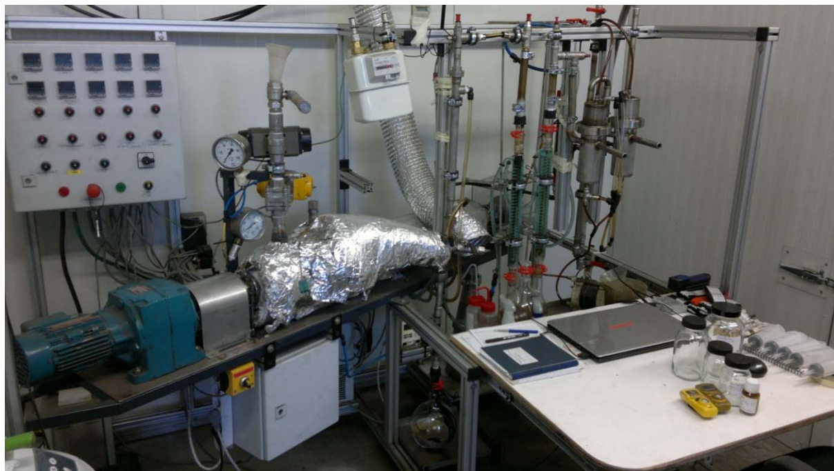
Figure 3 – BTG. Photograph of the torrefaction setup
