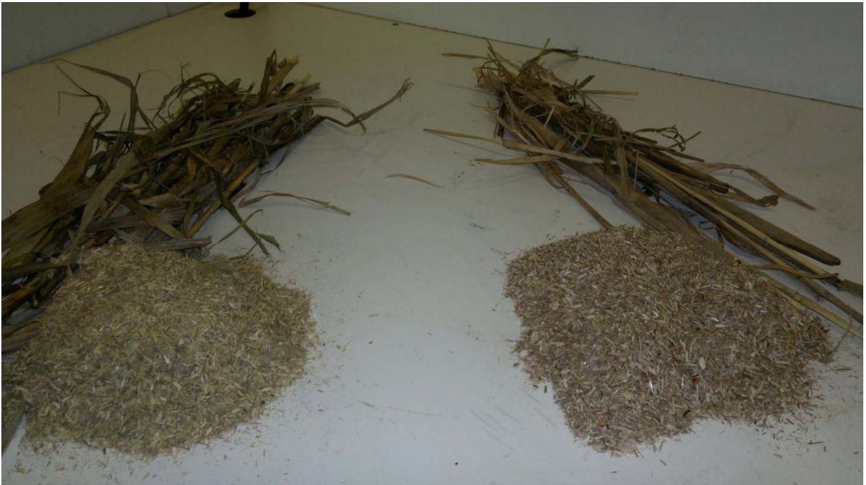
Figure 1 – BTG. photograph of the Arundo (left) and Miscanthus (right) biomass before and after size reduction.
