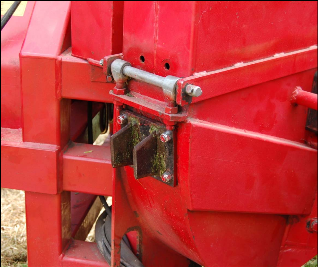
Figure 1 - SPAPPERI. Outer positioning of the counter-blades of the rotor.
