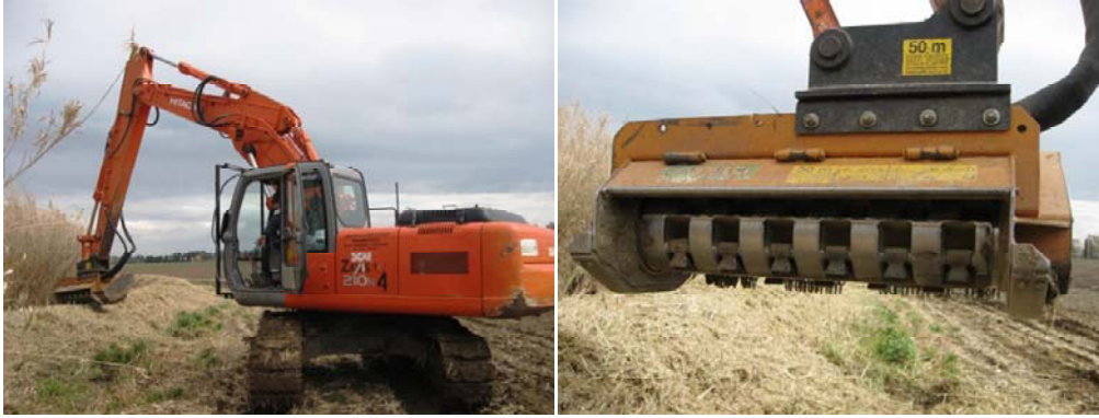
Figure 4 – CREA-ING. Hydraulic mulching head mounted on the tracked excavator
