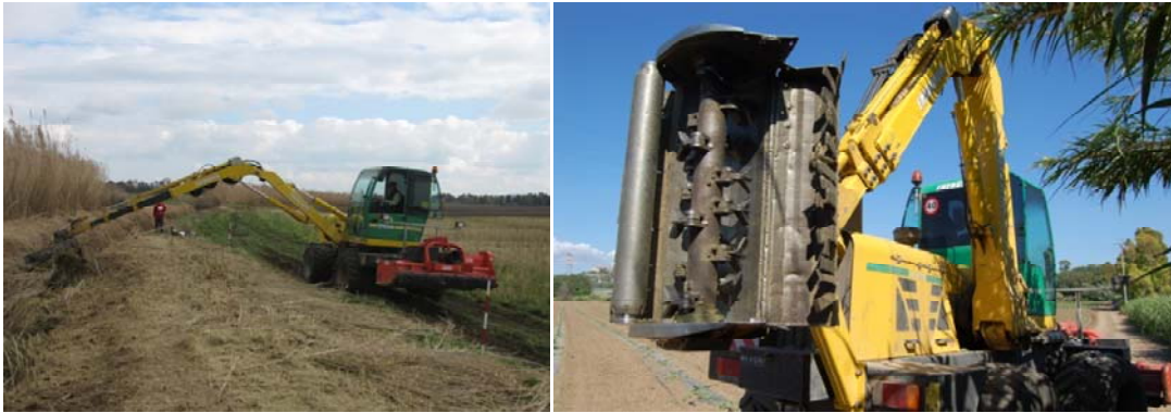
Figure 5 - CREA-ING. Shredder head with knives coupled with a self-propelled
