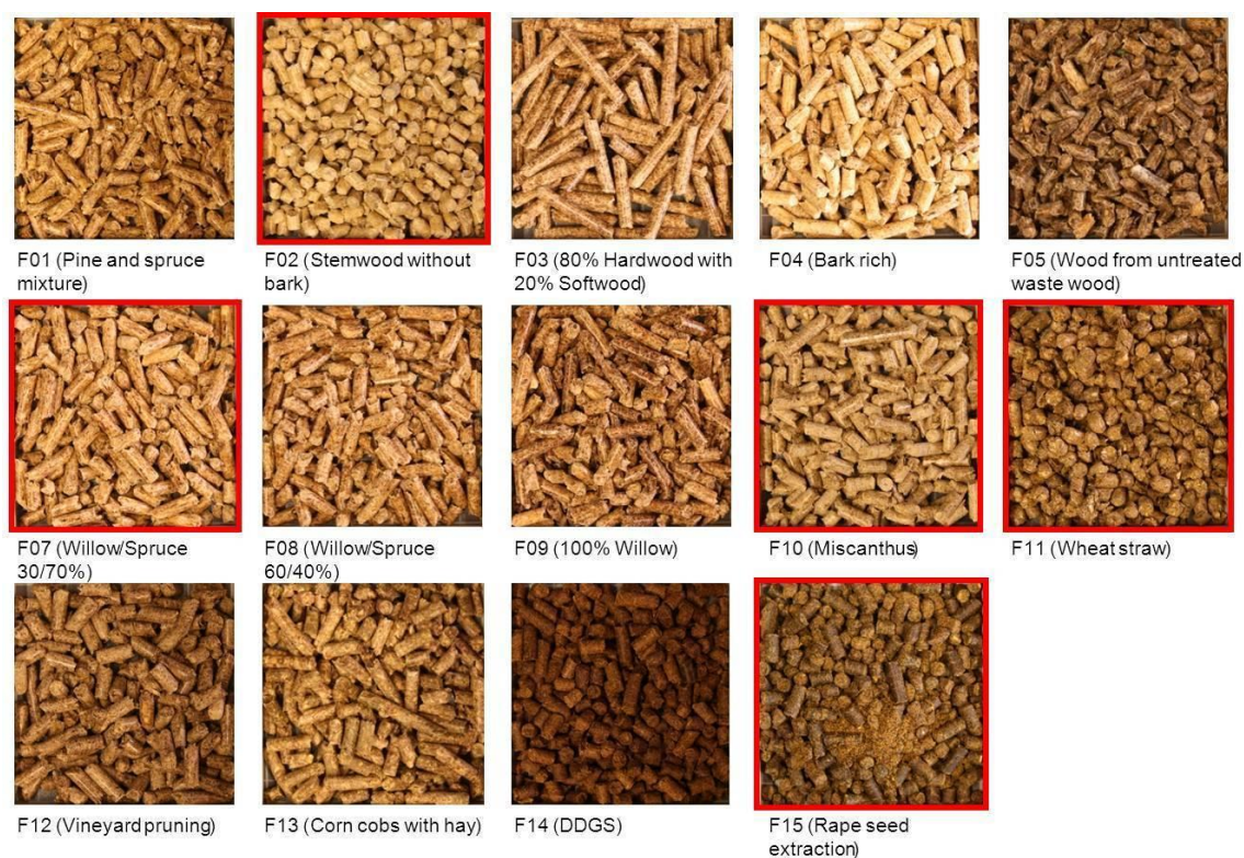
Figure 2: S&T results, Evaluation of laboratory tests - Fuels for laboratory tests (all pellets) and for boiler tests (pellets in red box) (source: TFZ)
