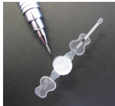
Produced parts with SONO”R”US technology: Medical and precision mechanic sectors
