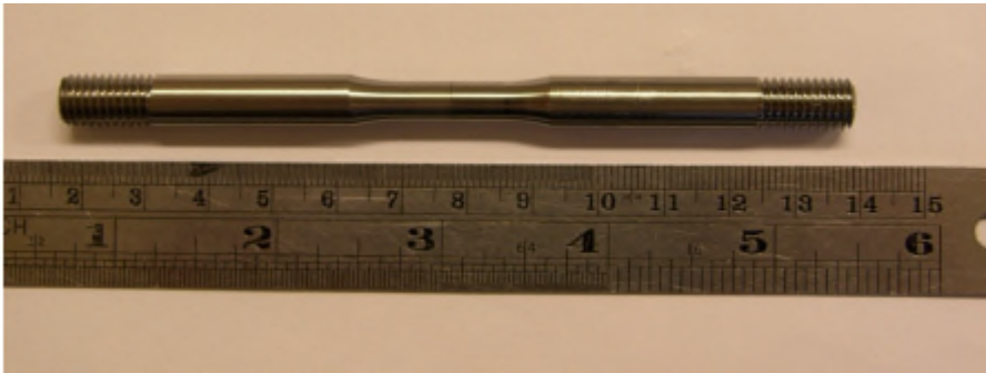
Figure 4: Fully machined TWI Test House tensile test sample (TWI Image)
