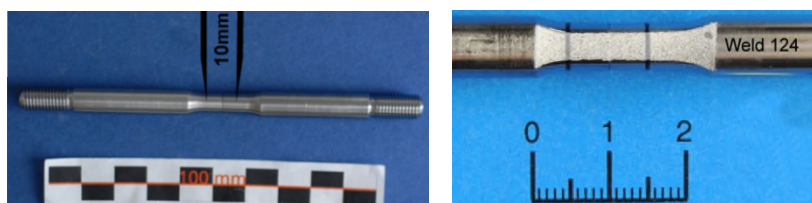
Figure 8: Tensile Test Specimen from Welds for Determination of the Local and Global Mechanical Material Behaviour of the Welded Area
