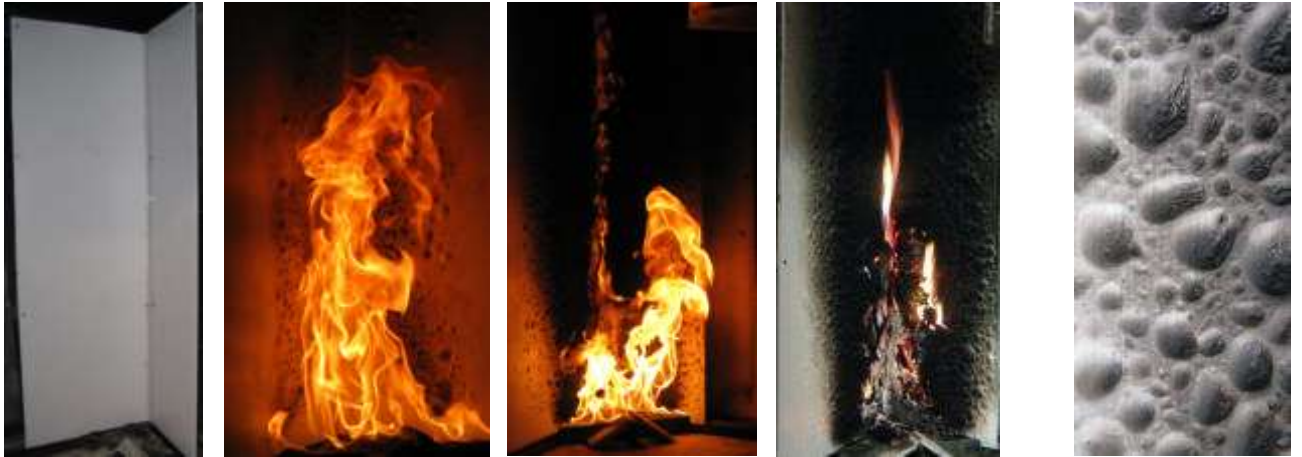
Figure 12. Furan-flax sandwich panel (as in Figure 11) coated with intumescent coating system (left) subjected to an SBI test (centre) showing surface intumescence after end of test (right).
