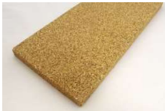
Figure 2. Resin bonded cork crumb panel from Amorim Cork Composites to be used as a core material
