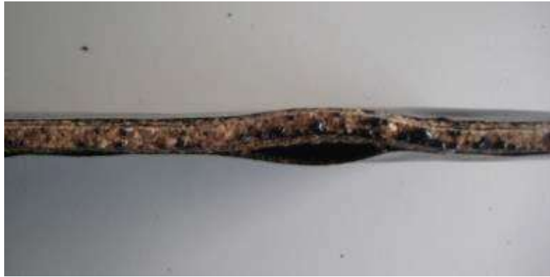
Figure 4. Result of a preliminary feasibility trial showing the effect of uncontrolled steam production during the cure of polyfurfuryl alcohol laminates with a cork core.
