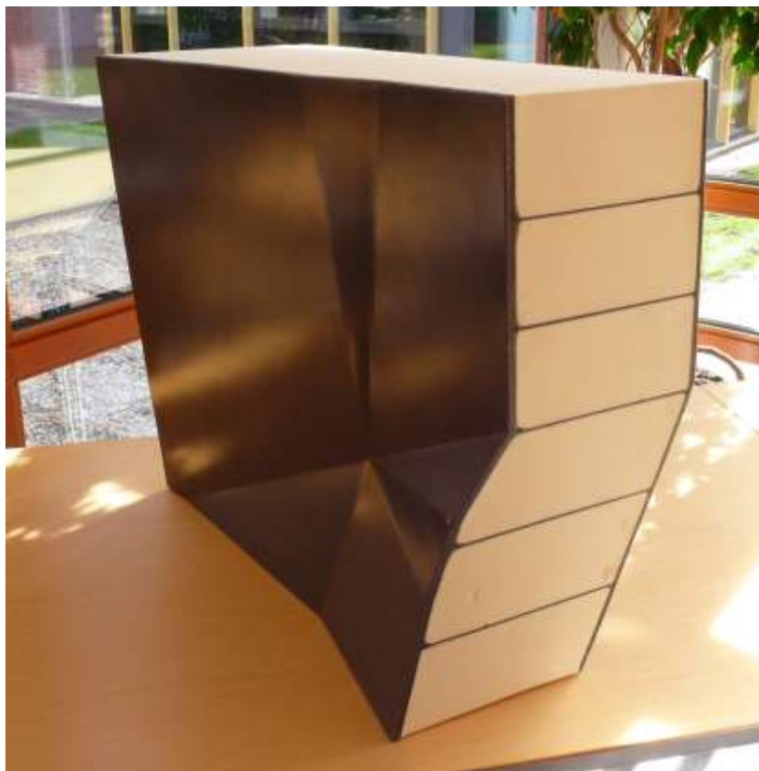
Figure 5. The first version of a small scale EWP. The later design used a loose fill insulation and the through thickness ribs were removed to reduce thermal bridging.
