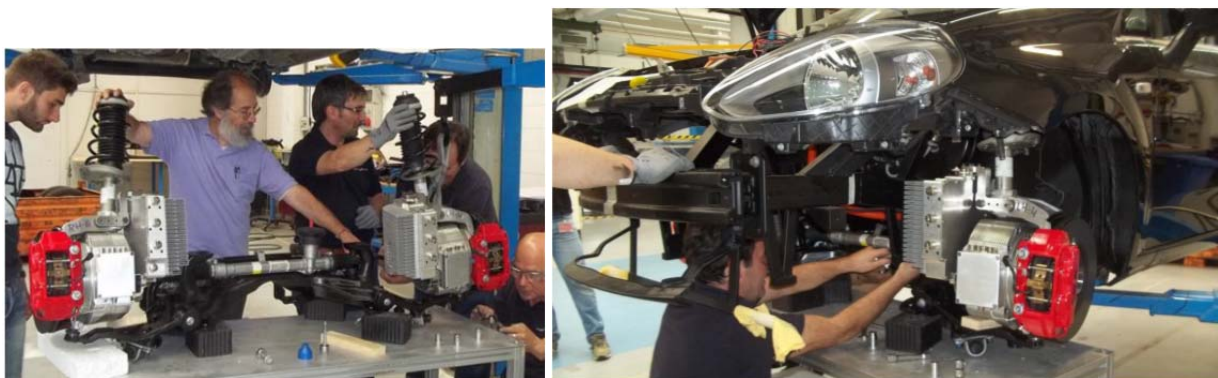
Figure 42: Final EUNICE in wheel system integration in donor car.
