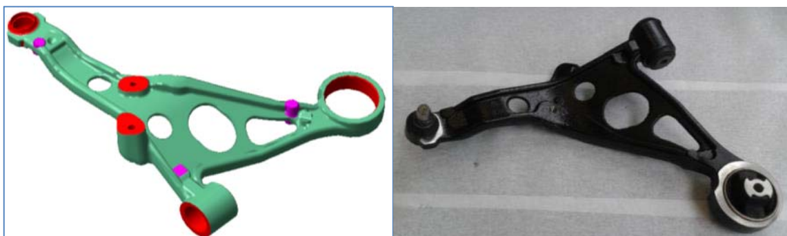
Figure 19: EUNICE suspension control arm CAD model and final prototype manufactured in cast iron with ADI heat treating process.
