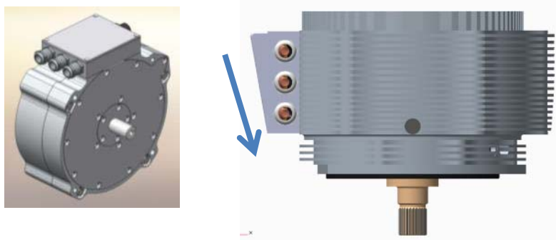
Figure 23: New connection box design to deflect the air to the gearbox
