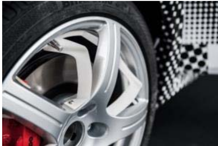
Figure 32: Final wheel rim prototype with aerodynamic blades to increase EUNICE motor in wheel air cooling performance.
