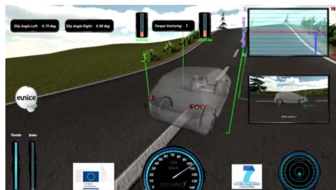
Figure 16: Tuning and validation of torque vectoring algorithm using virtual driving environment.
