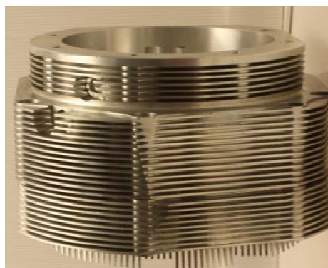
Figure 24: Electric motor finned outer case to improve heat transfer.
