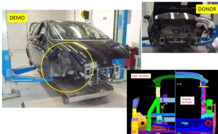
Figure 41: Final structural differences between donor and demo
