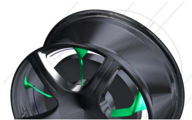
Figure 28: CDR Rim (grey) and new blade design (green)
