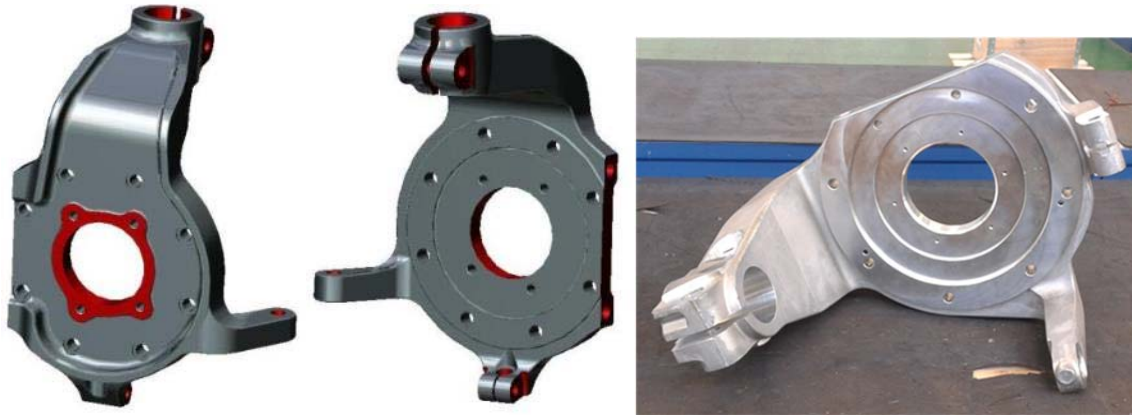
Figure 18: EUNICE suspension knuckle CAD model and final prototype manufactured in aluminium with low pressure die casting.
