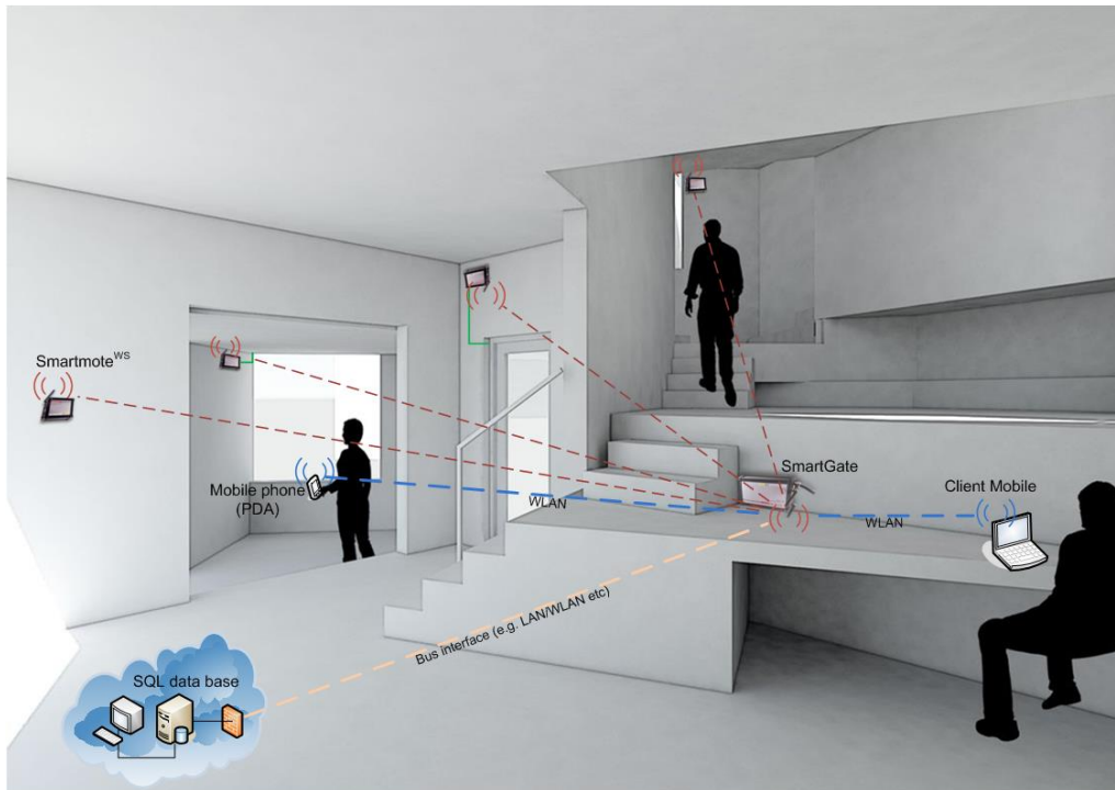
Figure 1: Principle sketch of the wireless sensor network system
