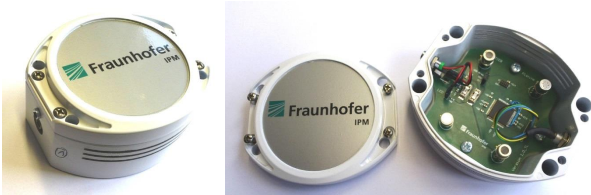
Figure 5: Left: Aluminum MOX sensor node box with integrated MOX sensors. Right: Open MOX sensor node with four MOX-sensors, PCB board and microcontroller.
