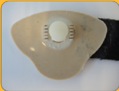
PP2. Textile cable and snap connector positioned for overmoulding (Synesis)
