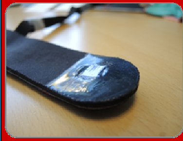
HR3. Coat sensors with silicone coating to protect and give better skin contact
