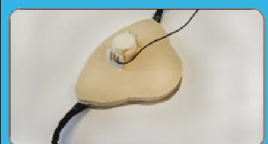
RR4. Overmoulding of UID silicone base (Synesis)
