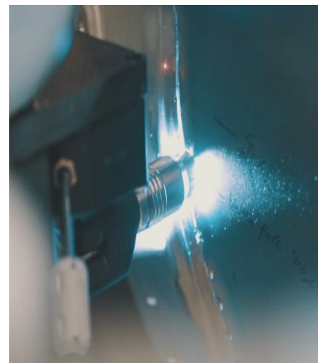
Figure 18: Automatic tack welding of the TRF at GKN
