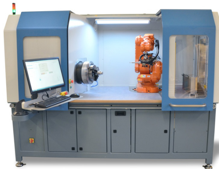
Figure 36: Strecon's Robot Assisted Polishing machine
