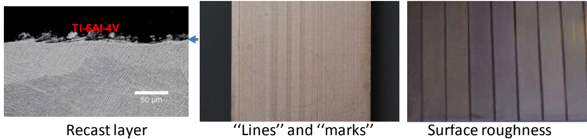
Figure 43: typical defects of wire EDM products
