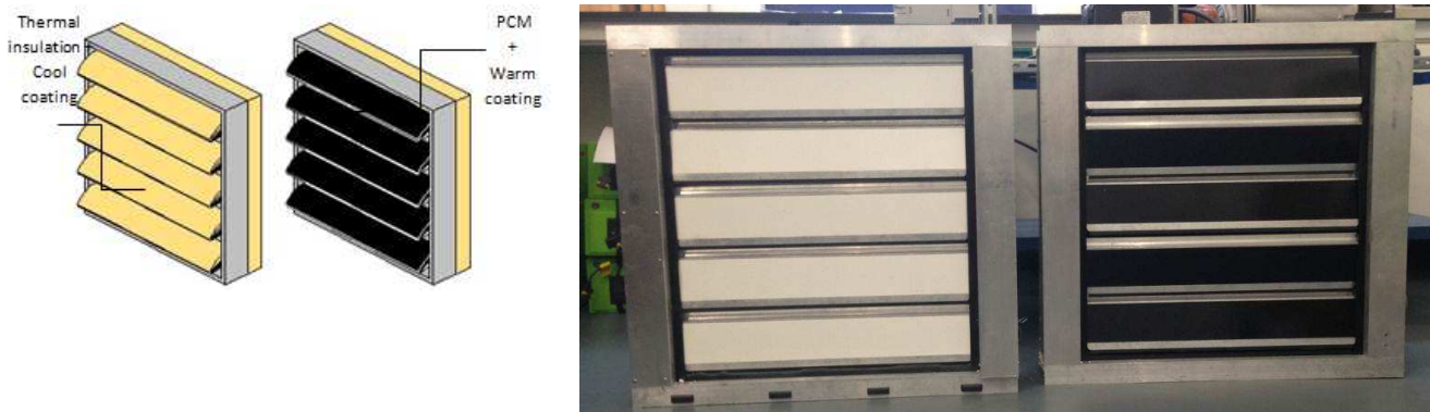
Figure10. Design concept and the first prototype on Advanced Passive Solar Protector and Energy Absorption Technological Unit
