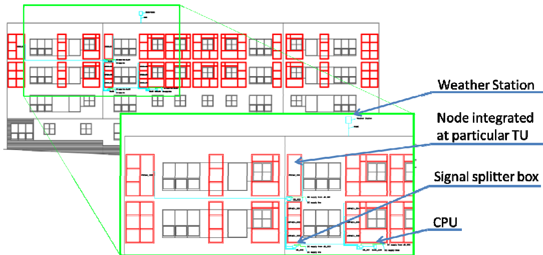
Figure 27. Overall layout of the Demo EMS structure
