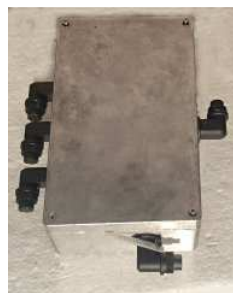
Control boxes (communication between CPU and TUs)
