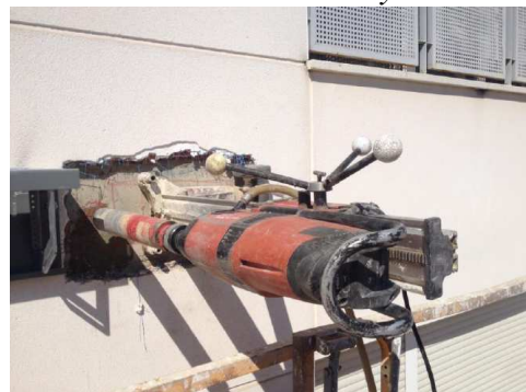
Figure 42. Traction tests performed and concret strength tests.
