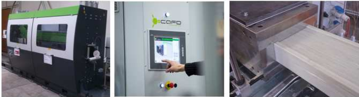
Figure 32. The novel prototype reactive thermoplastic pultrusion line.
