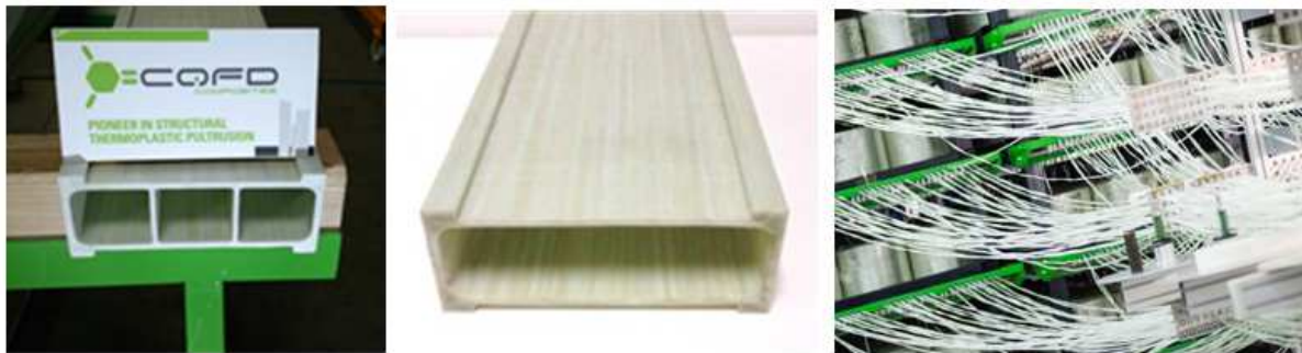
Figure 30. The large thermoplastic complex composite hollow cavities profile manufactured.
