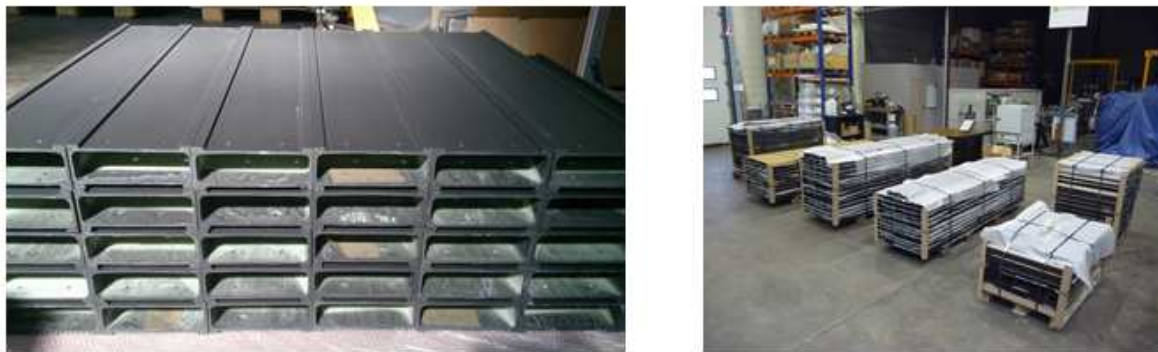
Figure 33. Special non-burning inorganic paint for thermoplastic composite profiles
