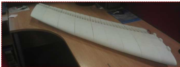
Wing equipped with honeycomb trailing edge.
