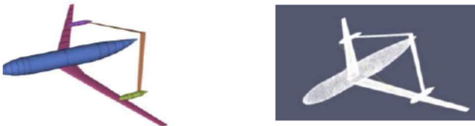
Figure 42. Joined Wing Regional Jet Designs Considered in this Study.
