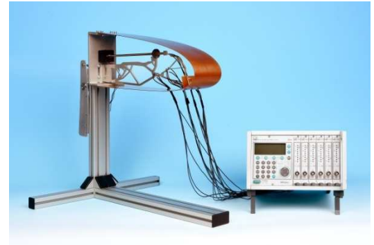
Figure 4. DLR benchtop droop-nose demonstrator designed, built and used as an intermediary step for the final morphing wingtip wind tunnel model.
