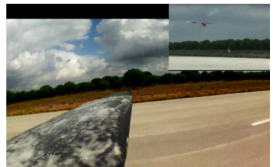
Figure 13. Telescopic wing of the RPV aircraft during landing.
