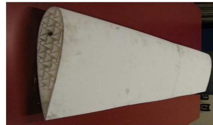
Wind tunnel model based on chiral structure
