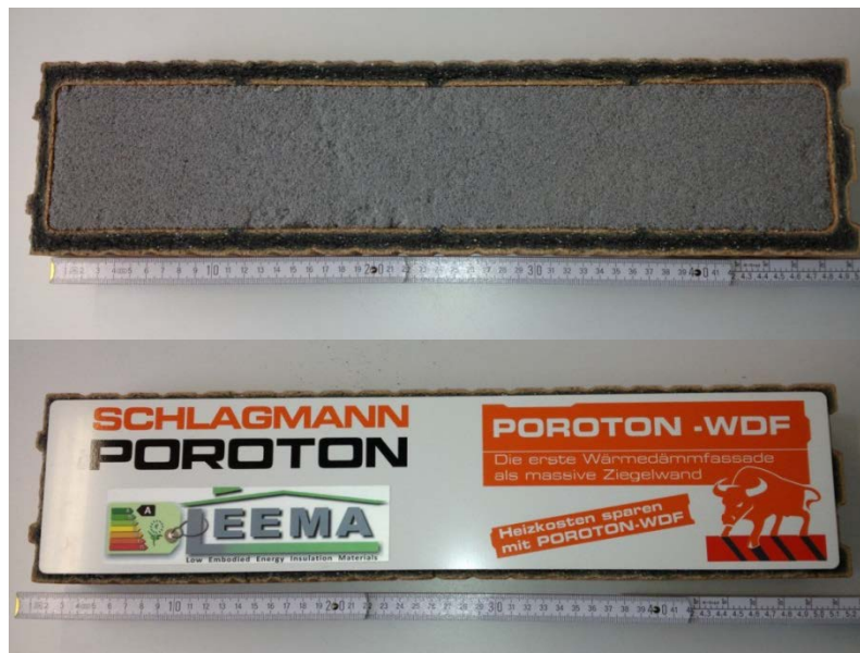
Figure 1.5. 3I Façade panel for refurbishment: “WDF”
