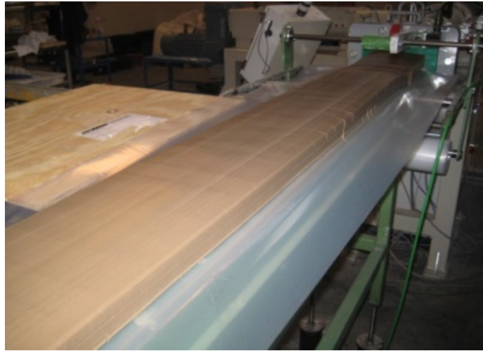
Figure 1.6. Extruded column of 3I binder
