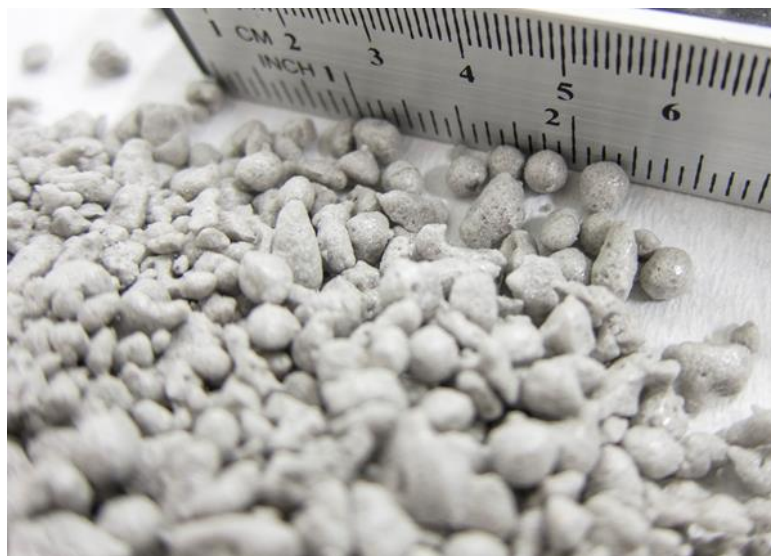
Figure 1.1. 3I Loose Filling materials for cavity walls
