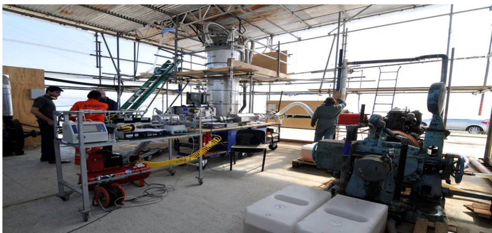
Figure 1 Pilot Scale system showing: Engine, PM monitor, Cooler, NTPR unit and ESWS
