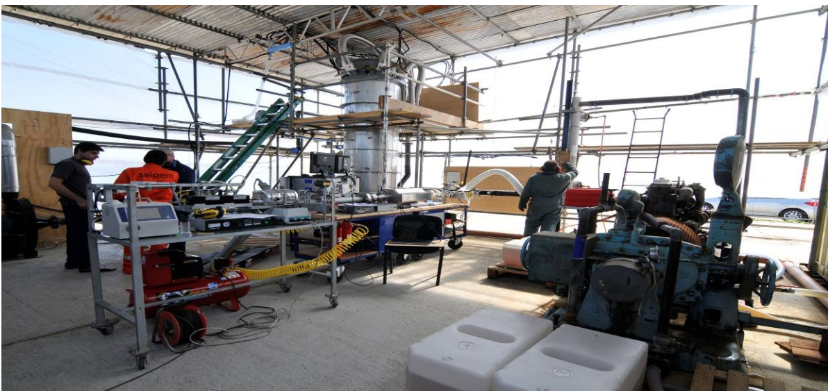
Figure 6 Pilot Scale system showing: Engine, PM monitor, Cooler, NTPR unit and ESWS
