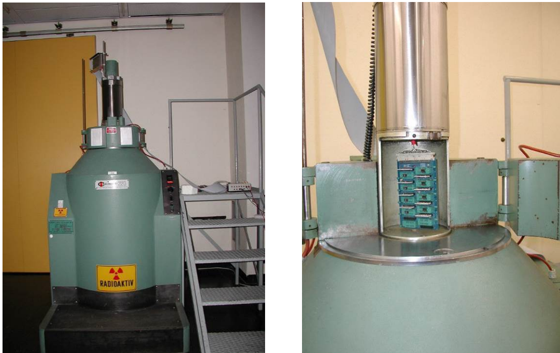
Figure 3-34 ^{60}\text{Co} Source for TID testing (left) and Cylindrical Chamber with an Example of a Test Board (right)
