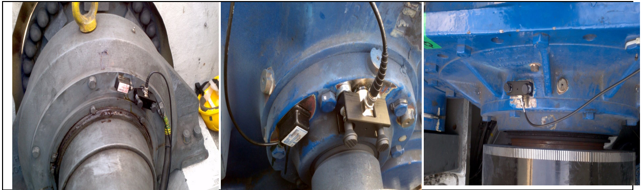
Figure 5 AE sensors (KH and Vallen) on main bearing (LHS), AE on high speed gearbox bearing (Middle) and AE on low speed gearbox bearing (Right)
