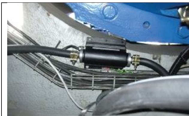
Figure 8 Oil sensor (left) and digital counter (right) installed on the NEG-MICON 750kW wind turbine at CRES's wind farm in Lavreotiki, Greece, the operational temperature range of the wear debris sensor is from -20°C to +65°C. The maximum permissible pressure of the oil is 10 bar
