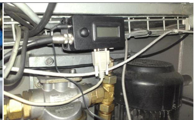
Figure 8 Oil sensor (left) and digital counter (right) installed on the NEG-MICON 750kW wind turbine at CRES's wind farm in Lavreotiki, Greece, the operational temperature range of the wear debris sensor is from -20°C to +65°C. The maximum permissible pressure of the oil is 10 bar
