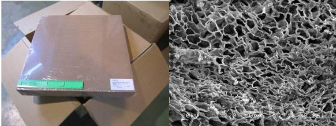
Figure 6 Norcoat panels: a) 1 panel 550 x 550 x 70 mm and b) Microstructural inspection at arrival
