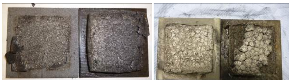
Figure 12: Fractured surfaces of C/C-SiC/NORCOAT/C-C-SiC joints: with Graphibond 669 (graphite) tested at 700°C LEFT, with Ceramabond 835 (ZrO 2 -ZrSiO 4 ) tested at 700°C-RIGHT.
