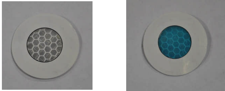
RFID Tag before (L) and after (R) exposure to Oxygen)
