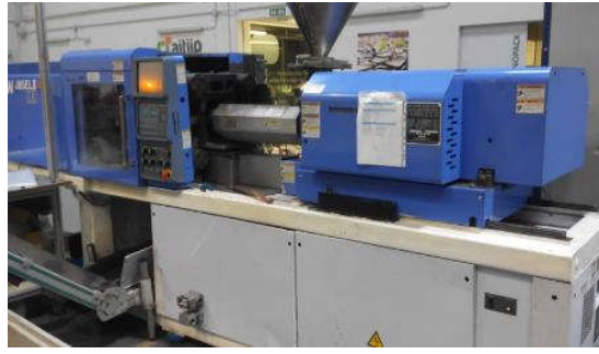
Figure 11. Peripherals It is expected to have a vacuum pump near the machine/mould in order to place the label on the IML system. Apart from that, no other external peripheral is expected.
