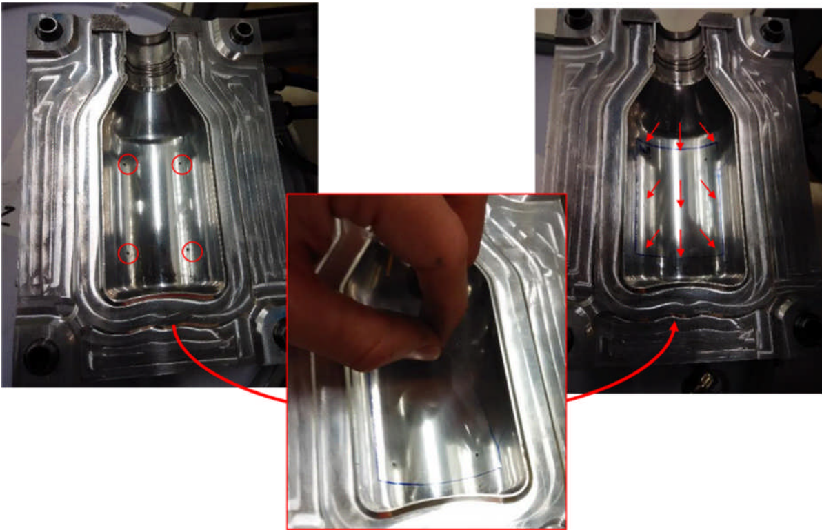
Figure 24. The constructed mould with the IML system operative
