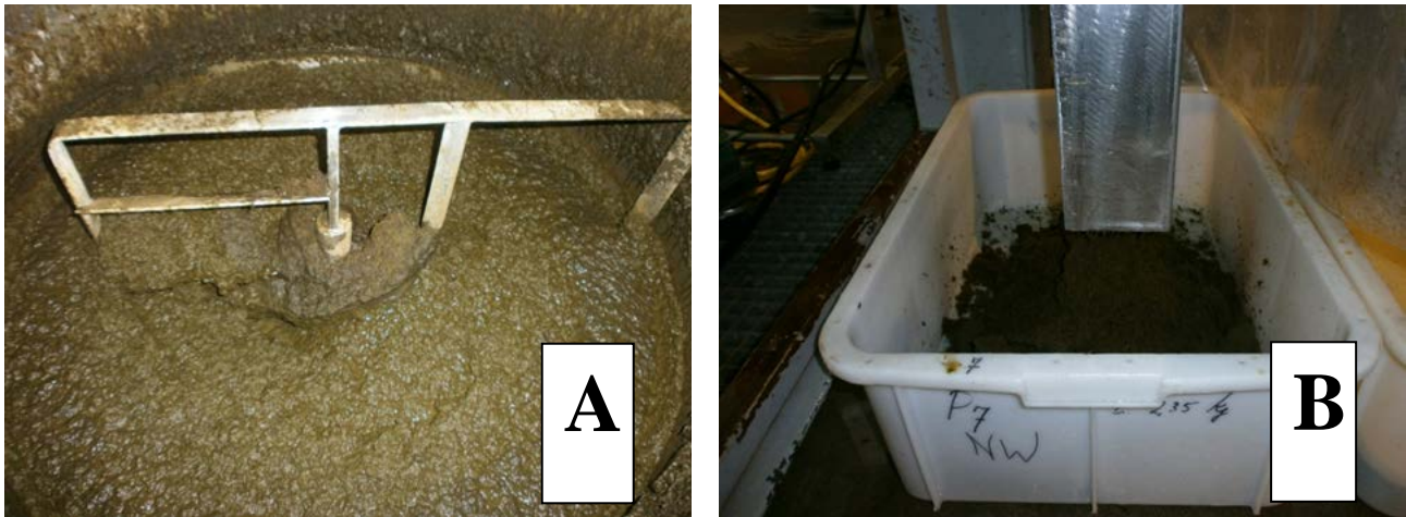
Fig. 5 Solid fraction of verge grass used for enzymatic hydrolysis. A: after extrusion and alkali treatment, B: the same after decantation. The decantation device uses centrifugal forces to separate water from solids.
