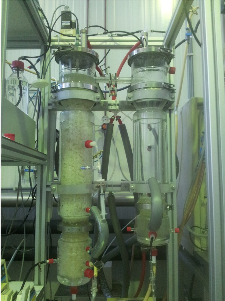
Fig. 7 Combined packed bed (left) with gas-disengager (right) (CFBG). The packed bed was filled with Bioflow 9 polyethylene carriers. The diffuser is at the bottom part with the floating balls. The working volume for the fermentation is 5.7 L
