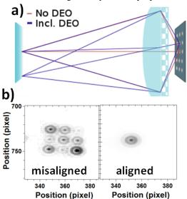
Figure 1 A network of VCSELs. Panel a) shows the principle mechanism of coupling between lasers. Without the DOE, each laser forms a single image on the SLM. Including the DOE (checker-board patterned element) results in the creation of multiple images per laser due to diffraction, overlapping for neighbouring lasers. Panel b) demonstrates the coupling for different angles (+6 and 0 degree), and an image of the intensity caused by the feedback coupling from
