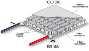
Static thermoelectric converter (TEC) module
