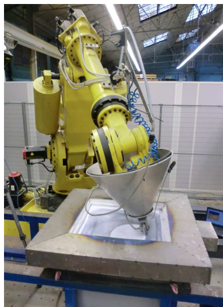
Asymmetric incremental forming robotic cell
