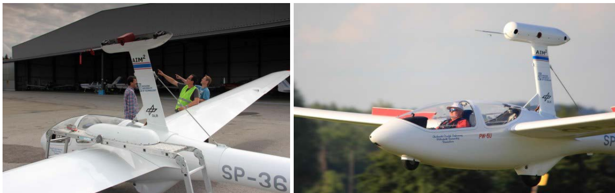
Figure 16: Camera pod on the PW-6 glider (left - pod opened for camera adjustment on ground, right - PW-6 glider with pod flying)
