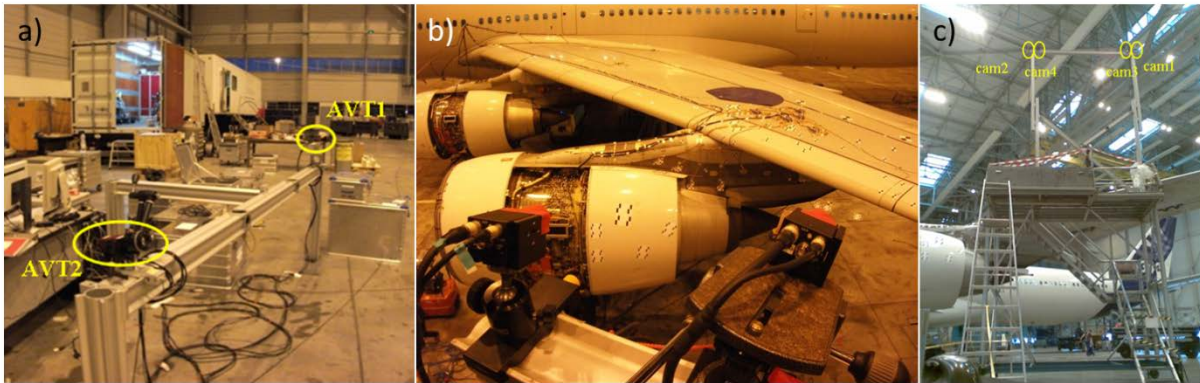
Figure 3: The GVT on an A340 chosen for the evaluation in Task 2.3 ( a - high resolution cameras on ground observing the nacelle, b - observed wing and nacelle with markers, c - position of the JAI camera systems)
